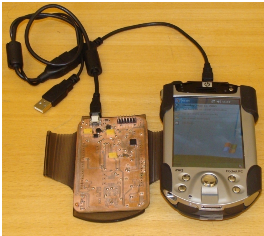
Figure 41: Connecting the Wasa board to the HP iPAQ PDA
