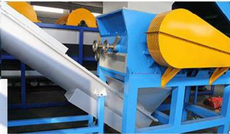
screw conveyor from crusher to floating washer
