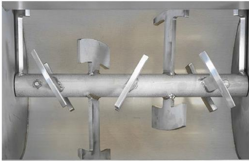
77-PV0077/C Detail of drum with helical mixing shaft
