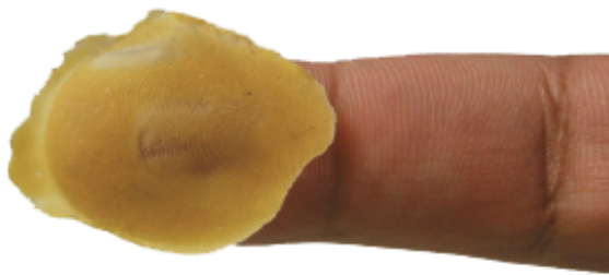
Figure 3.1: Fingerprint spoofing: Wafer-thin plastic sheet housing a three-dimensional replication of a fingerprint. Image found in [29].
