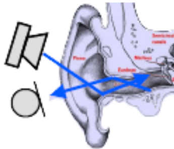
Figure 4.4: Functionality of acoustic ear recognition: A sound signal is probed into the ear which is reflected and picked up by a microphone, thereby generating an ear signature. The figure is found in [1].
