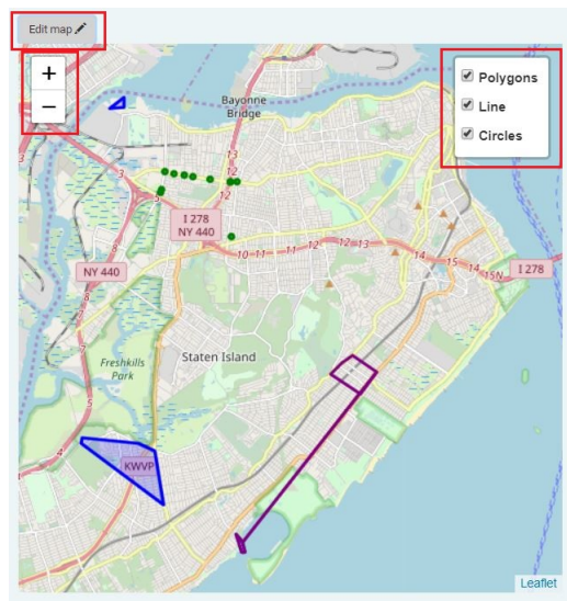
Figure 5.13: The map container contains the "edit map" button and the map itself. Here displayed with the zoom tool (top left corner) and a open layer controller (top right corner). Figure 5.12 displays a closed layer controller
