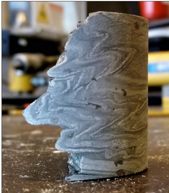
Figure 5.19: Typical mode of failure for axial point load tests on specimens from block 2.
