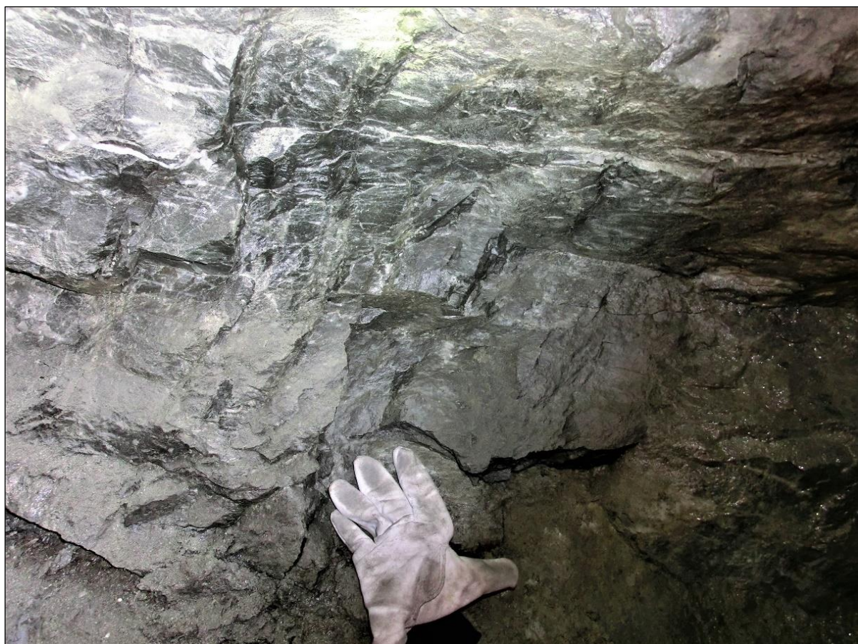
Figure 5.2: Photo of the rock mass in the niche at chainage 430 of the R1. The rock is a greenish grey, fine-grained metasandstone. Glove for scale.
