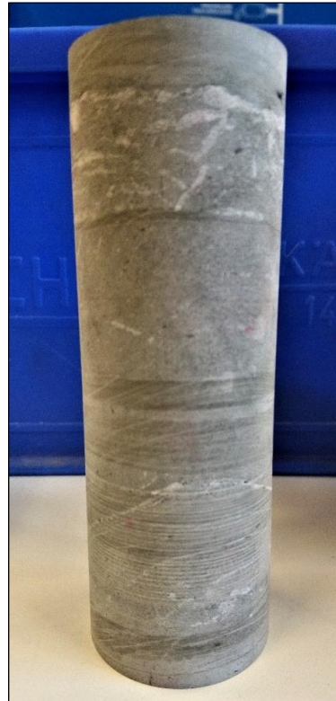
d) Specimen from block 4: similar to block 1, with additional dark bands
