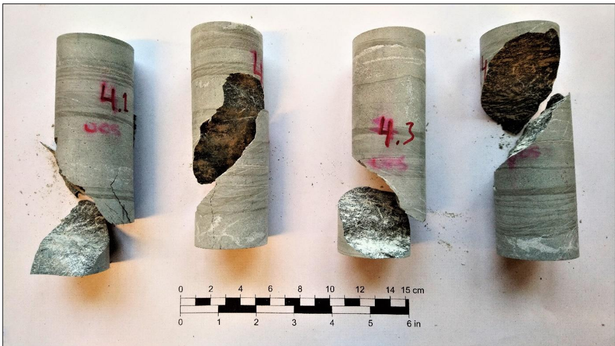
Figure 5.18: Photo of specimens 4.1–4.4 (from left to right) after the uniaxial compression tests. The specimens have generally failed in shear along surfaces influenced to various degrees by a second foliation.
