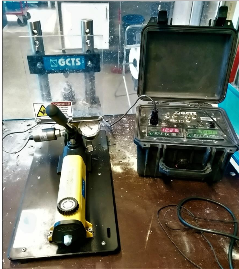
Figure 5.11: The GCTS PLT-100 Point Load Test System, used for point load testing in the laboratory.
