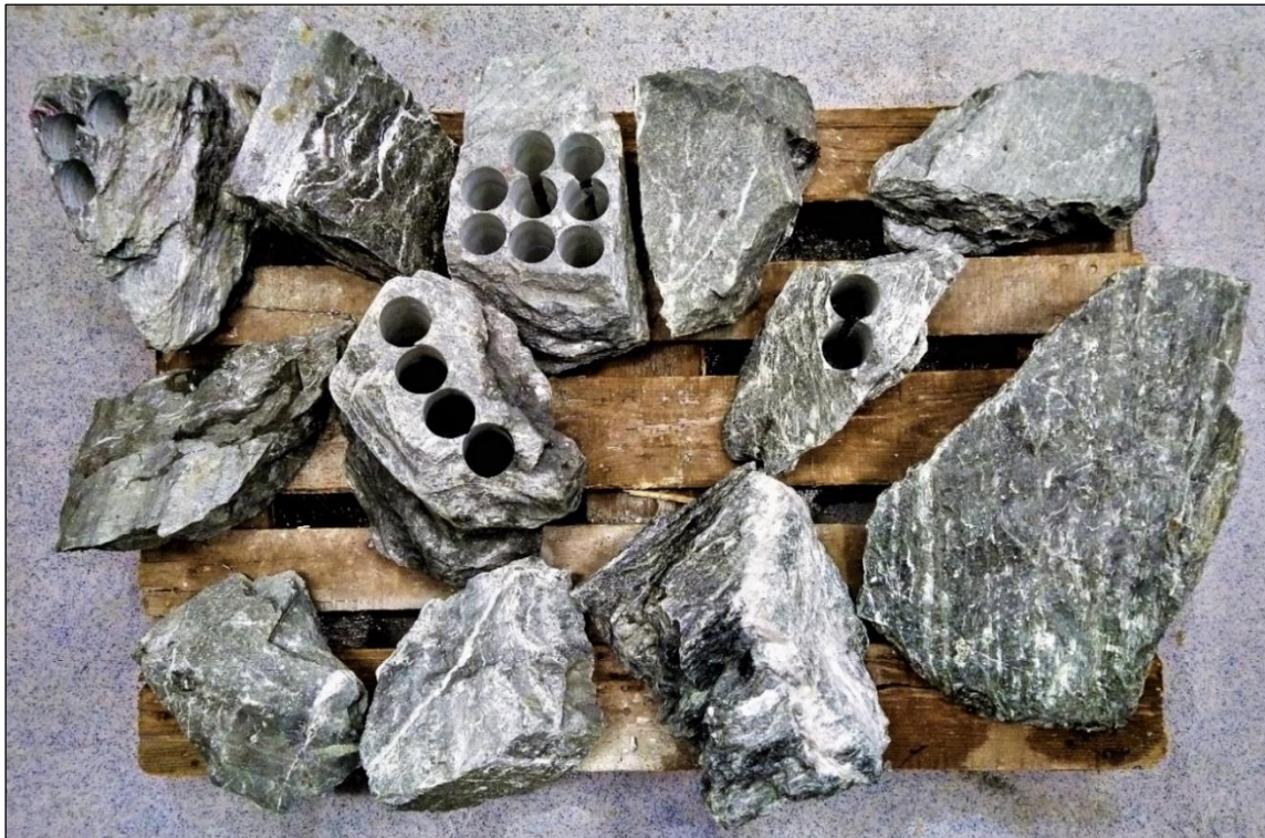
Figure 5.9: Blocks collected from the R1 for use in laboratory investigations. The four blocks that were used are the ones from which core specimens have been drilled. From left to right: block 2 (three cores), block 4 (four cores), block 1 (eight cores) and block 3 (two cores).
