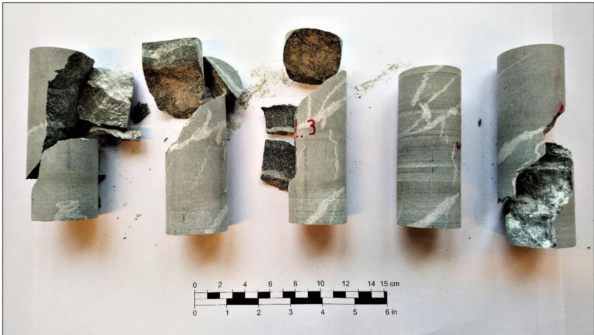
Figure 5.17: Photo of specimens 1.1–1.5 (from left to right) after the uniaxial compression tests. The specimens have generally failed in shear along surfaces influenced to various degrees by a second foliation. Specimen 1.3 failed in a combination of shear and axial cleavage. Note the scarcely visible failure surface down the centre of specimen 1.4.
