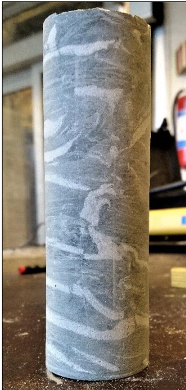
c) Specimen from block 3: metasandstone with quartz bands in a chaotic pattern
