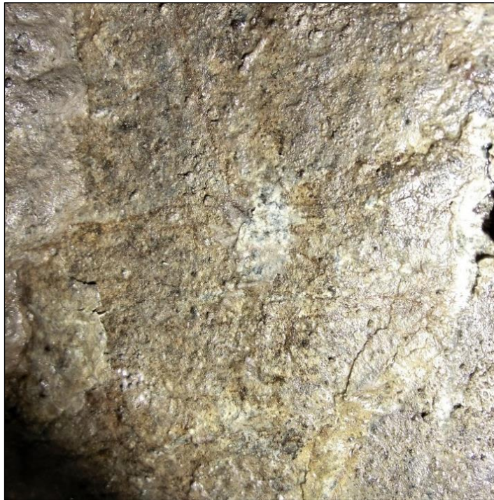
b) After testing (detail view). The impact point is seen as a white mark.
