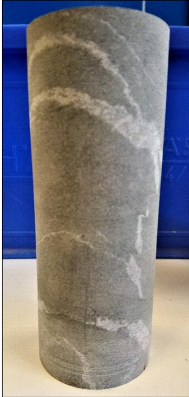
a) Specimen from block 1: pale grey, fine-grained metasandstone with quartz bands
