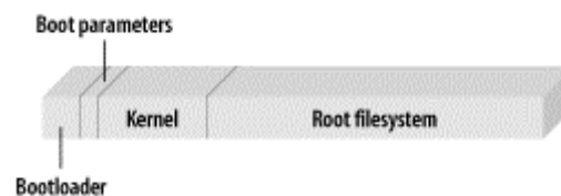
Figure 15: The solid-state media configuration [7]
