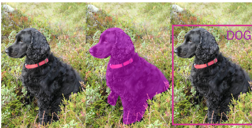
Figure 3.14: Difference between segmentation (Middle) and Object Detection (Right). The semantic segmentation mask is denoted with a pink mask, while the object detection bounding box is shown with a pink box together with the identified class.
