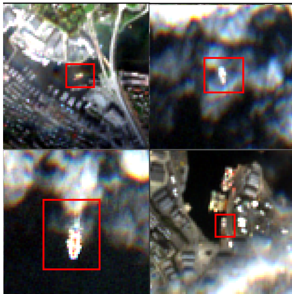
Figure 3.8: Four examples of ships incorrectly identified when using F-Mask cloud masks.
