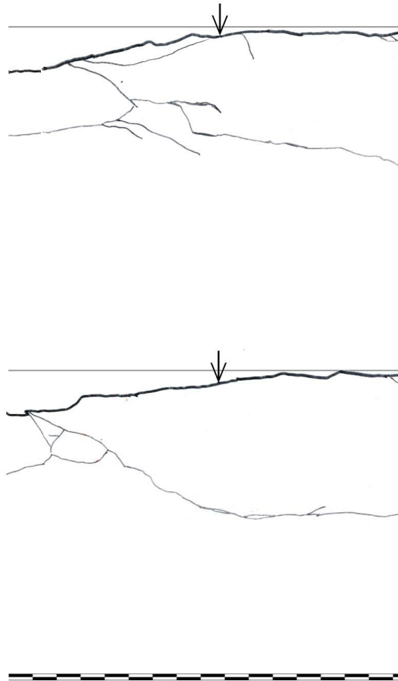
Figure I1.41: Surface and crack pattern under the cutter groove in core sample R_5458_1-3_23.
