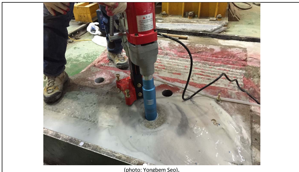
Figure E1.1: Sampling after linear cutter test with cutter spacing 80 mm. Note that the sampling was done from the bottom of the specimen
