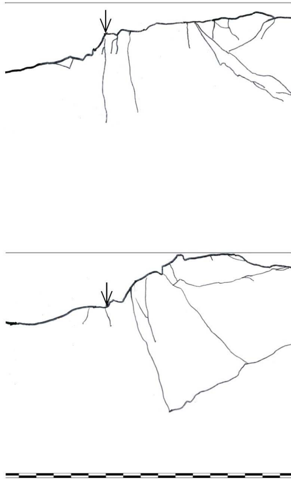
Figure I1.34: Surface and crack pattern under the cutter groove in core sample R_5437_3-4_25.
