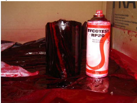
Figure 4.26: A) Application of penetrant. B) Core sample after application of developer, but before the cracks were fully developed.
