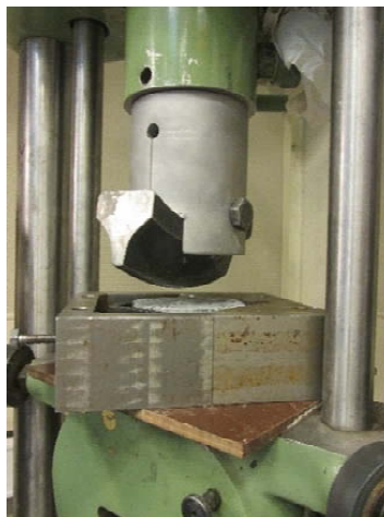
Figure 4.23: Apparatus used to partially clove the core sample.
