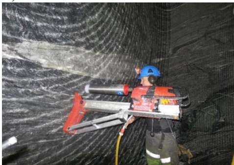
Figure 4.4: A) Core drilling into the face of the Nedre Røssåga headrace tunnel. B) Picture showing a typical sampling pattern.
