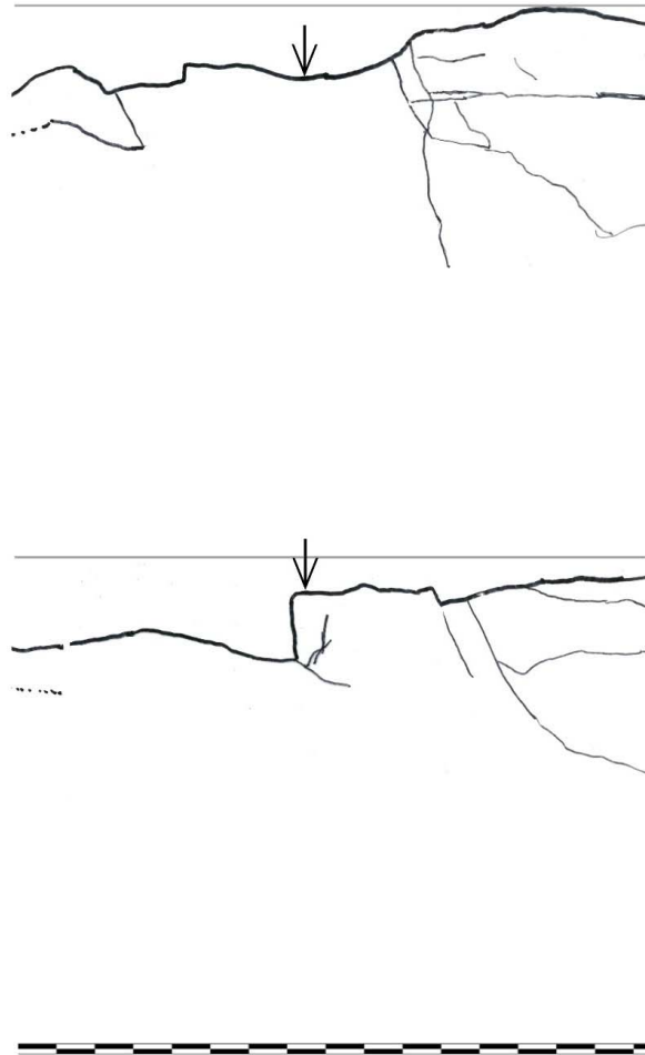
Figure I1.51: Surface and crack pattern under the cutter groove in core sample R_5458_4-1_21.
