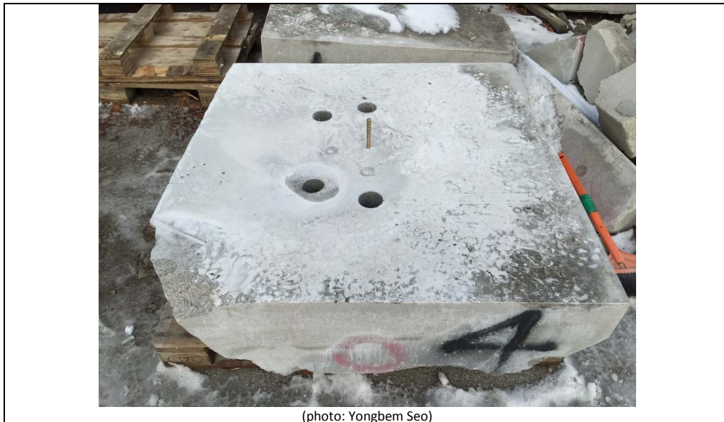
Figure E1.6: Sampling after linear cutter test with cutter spacing 100 mm. Note that the sampling was done from the bottom of the specimen.
