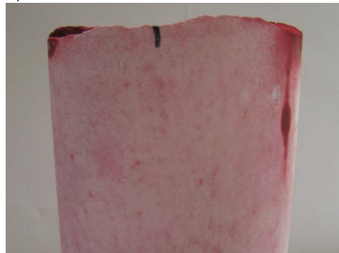
Figure 4.26: A) Application of penetrant. B) Core sample after application of developer, but before the cracks were fully developed.
