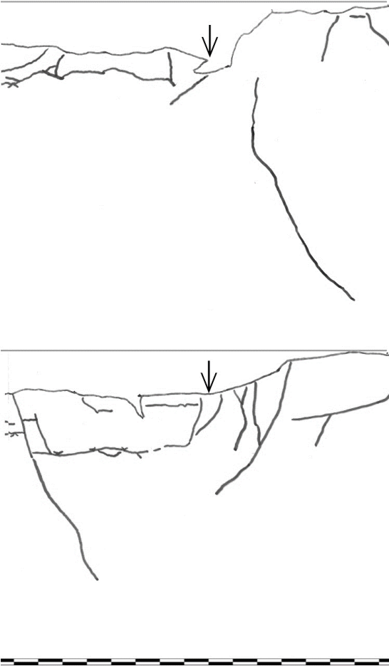
Figure I1.22: Surface and crack pattern under the cutter groove in core sample R_3112_6-1_37.
