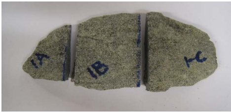
Figure 4.15: A) The chosen chips before cutting. B) Chip from the Nedre Røssåga headrace tunnel, chainage 1184. C) Chip from the AMR Project, chainage 11576.
