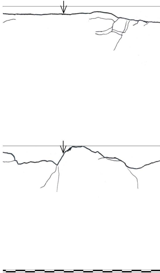
Figure I1.25: Surface and crack pattern under the cutter groove in core sample R_5437_1-3_23.
