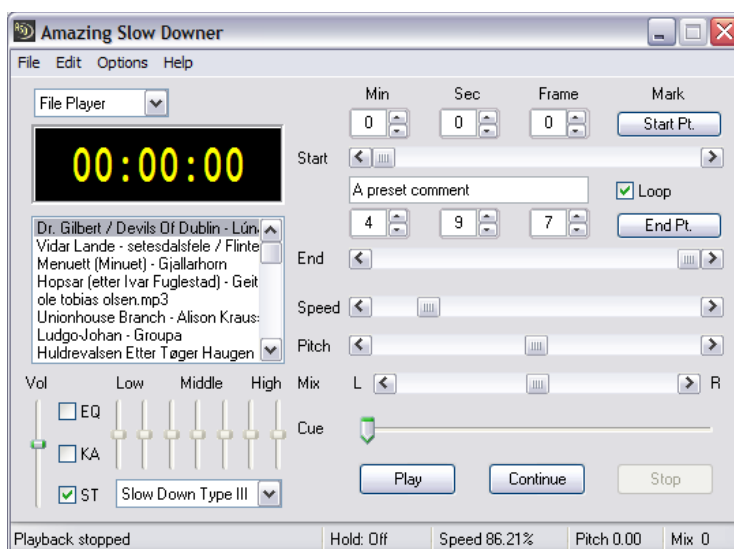
Figure 16: Amazing Slow Downer is an example of software that lets the user change playback pitch and speed independent of each other.
