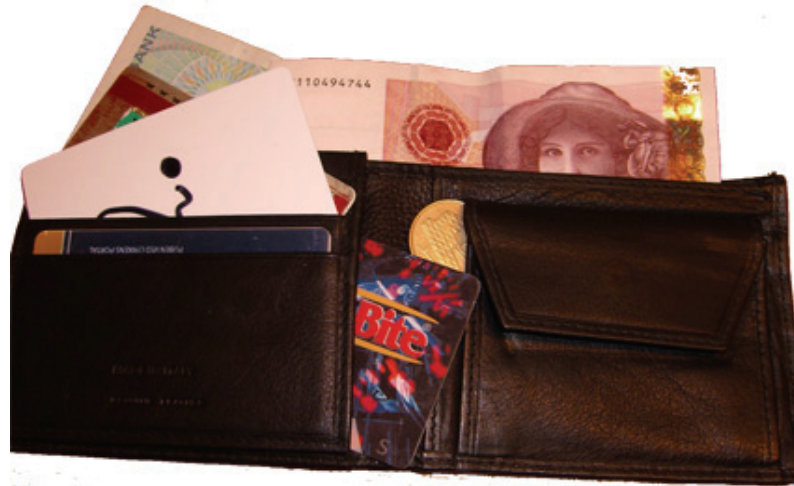
Figure 18: Leather wallet with content tested as a Faraday Cage
