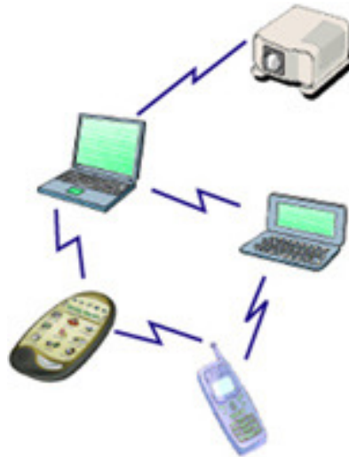
Figure 20: An illustration of a small ad-hoc network. Worth noting is the fact that there is no predefined infrastructure. Because of this nodes are expected to behave as routers and take part in discovery and maintenance of routes to other nodes.
