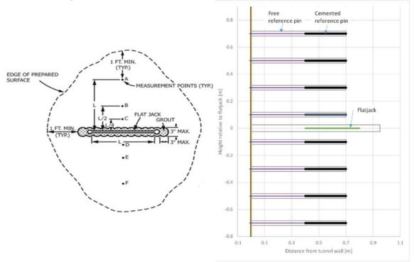
Figure 1. Flatjack array (left) according to ASTM (2008) and modified vertical section of the tunnel wall showing location of flatjack and measurement pins installed in a shotcrete lined tunnel (right).
