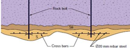
Figure 2. Schematic sketch of Reinforced Rib of Shotcrete.
