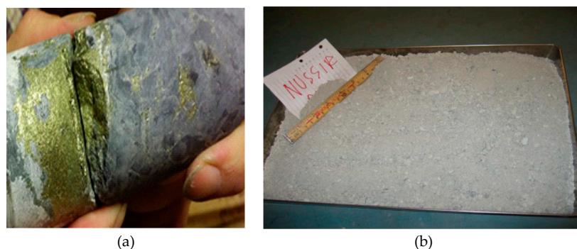
Figure 1. (a) The Nussir drill hole specimen: Veinlets of chalcocite and bornite on a carbonate structure; (b) the crushed ore sample received from Nussir ASA.
