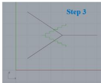
FIGURE 69) CODE IN GRASSHOPPER WITH VISUALIZATION OF EACH STEPS. STEP 1) IDENTIFYING THE INTERSECTION POINT AND THE ASSOCIATED INTERSECTION MEMBERS STEP 2) DEFINING “MASTER” AND “SLAVE” 3) CREATE A 2D INTERLOCKING PARAMETRIC “STAIR” 4) EXTRUDING THE GEOMETRY INTO A INTERLOCKING SURFACE
