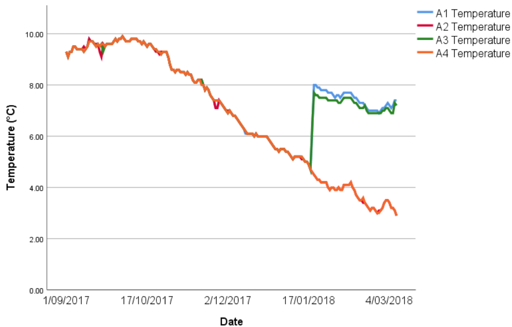
Figure 8. Temperature changes in the tanks over the course of the pilot experiment. Temperature (°C) shown on the Y – axis and time is shown on the X – axis. The peaks shown after the 17 th of January in tanks A1 and A3 represent the change from ambient water temperature to ambient +3°C.
