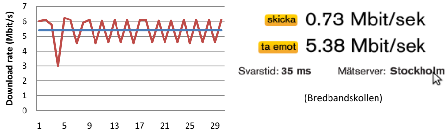
Figure 9.7: Bandwidth sampling (1 second interval) of ADSL (left) and reported values from Bredbandskollen (right).
