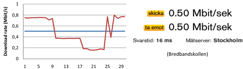
Figure 9.5: Bandwidth sampling (1 second interval) of Wi-Fi (left) and reported values from Bredbandskollen (right).
