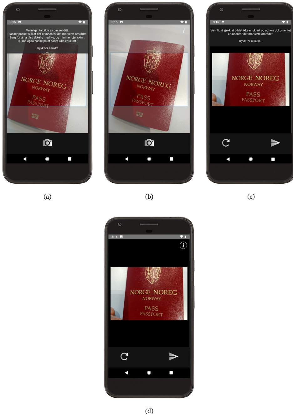
Figure 35: shows how the GUI of the camera is implemented for document photos. (a) shows how an information window provides the user with information regarding the photo. Both (a) and (b) provides a document border to where the document should be within. (c) allows the user to review the photo, and provides information as to some regular flaws with the photos.
