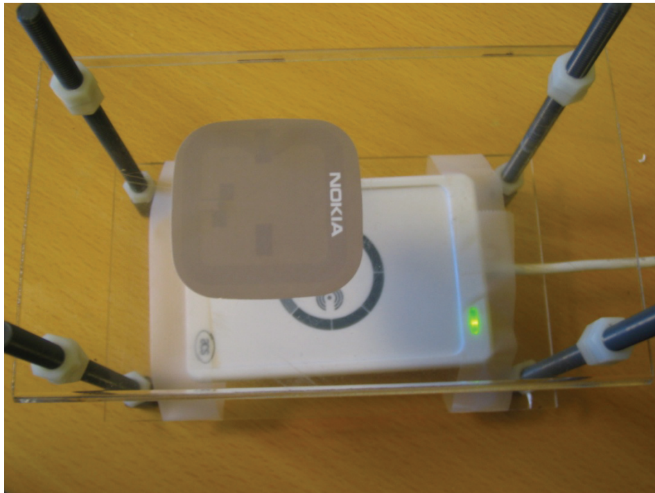
Figure 18: Reading range test set-up.
