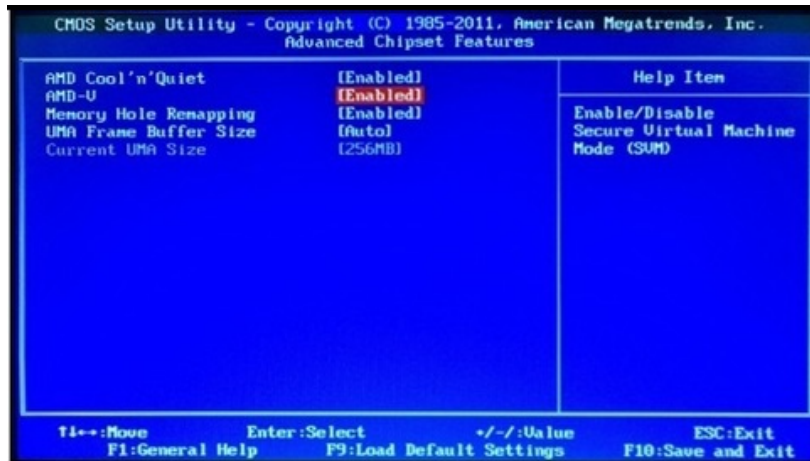
Figure 4.9: AMD SVM-Parameter in the original BIOS 11
