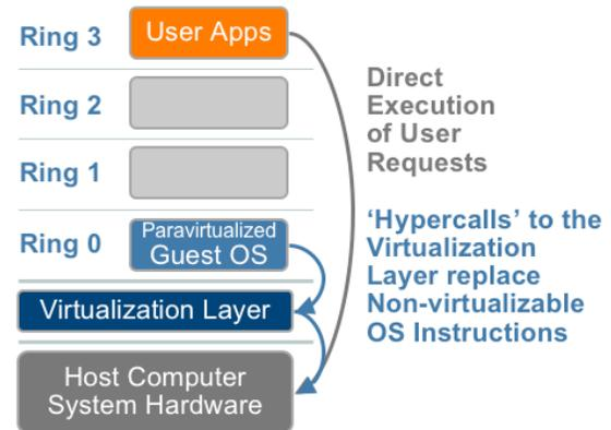
**Figure 6 – The Paravirtualization approach to x86 Virtualization**
