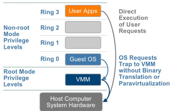
**Figure 7 – The hardware assist approach to x86 virtualization**
