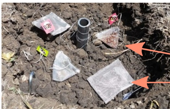
Fig. 1 A picture of the example plot setup: One excluded and one open litterbag of each litter type (four litterbags in total) in a \sim 20\text{cm}^2 and \sim 8\text{cm} deep hole.
