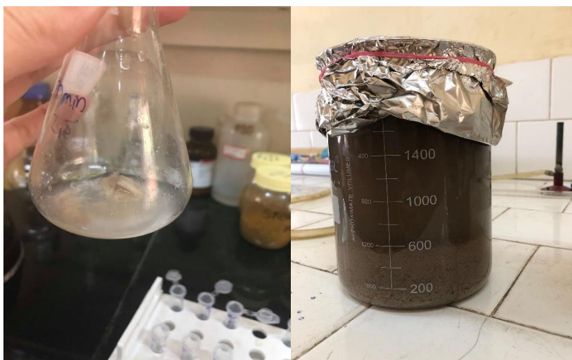
Figure 17: Steps in performing enzymatic hydrolysis at CFTRI Left: one of the conical flasks before enzyme was added displaying chunks of raw material. Right: After hydrolysis (Photos: Larsen, 2019)
