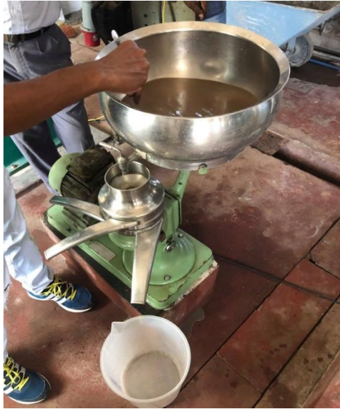
Figure 18: Separator used to remove the oil (Photo: Larsen, 2019)
