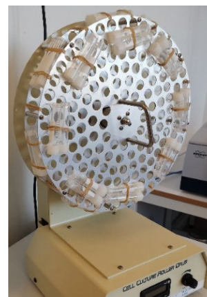
Figure 8. Setup of the end-over-end mixer.
