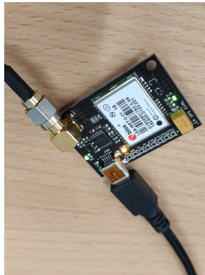
Figure 3.4: A NEO-M8T receiver (midlertidig)
