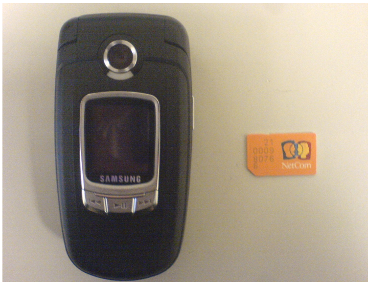
Figure 3.1: The Subscriber Equipment consists of the Mobile Station and a SIM card.
