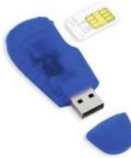
Figure 3.8: Equipment that can be used for connecting a SIM Card to a computer without a built-in SIM Reader
