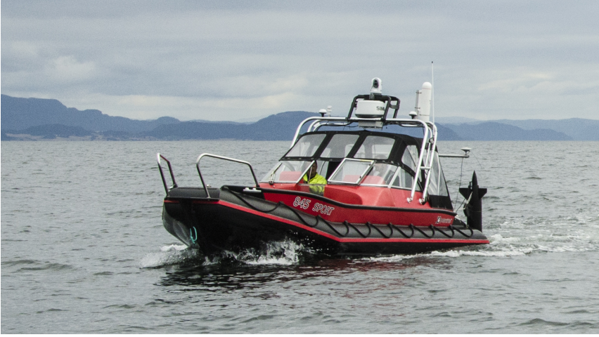
Figure 3: The Telemetron ASV, designed for both manned and unmanned operations. Courtesy of Maritime Robotics.
