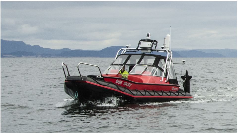
Figure 1.2: The Telemetron ASV, an 8.45 m long dual-use vessel designed for both manned and unmanned operations. Courtesy of Maritime Robotics.
