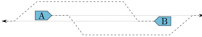
Figure 2.2: An example of a head-on situation, and how it can be solved by both vessels maneuvering to starboard.
