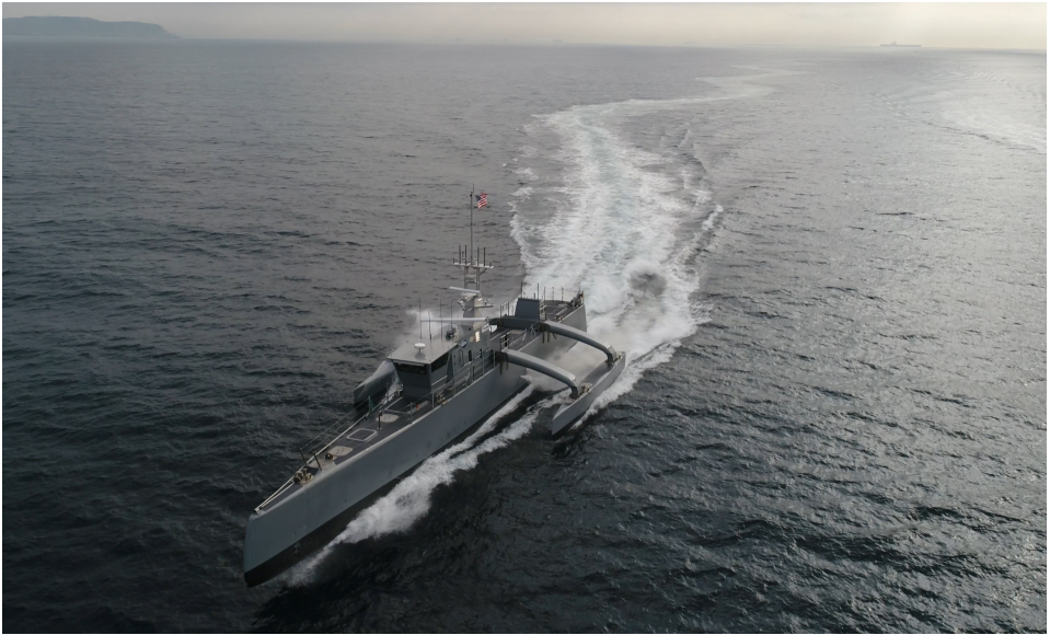
Figure 1.1: DARPA's Sea Hunter at sea tests in February 2017. The Sea Hunter is a 132-foot long ASV designed for detecting and tracking submarines for time periods over weeks or months [8]. Courtesy of Defense Advanced Research Projects Agency (DARPA).
