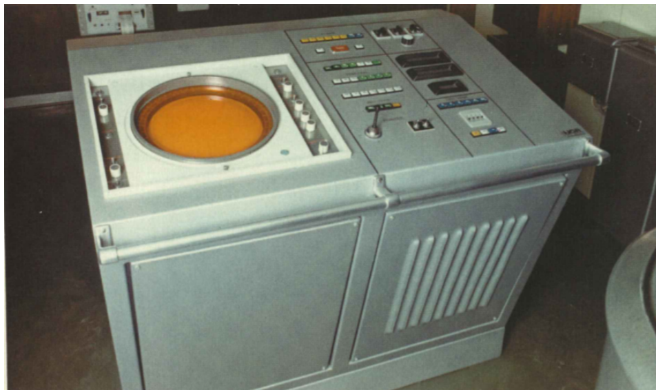
Figure 2.5: The prototype of the Norcontrol DataBridge installed on board the M/S Taimyr in 1969. Courtesy of Bjerva [58].
