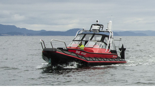
Fig. 1. The dual-use Telemetron ASV, which is 8.45 m long and capable of speeds up to 18 m/s. Courtesy of Maritime Robotics.
