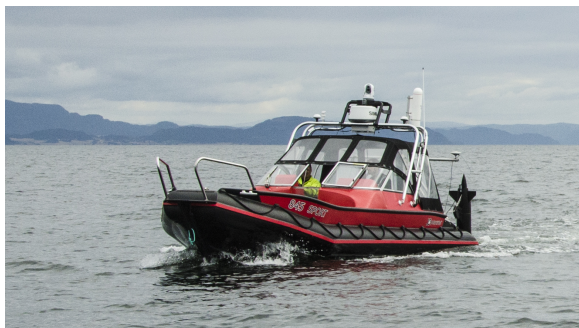
Fig. 1 The Telemetron ASV, which is a Polarcirkel Sport 8.45 m long dual-use ASV capable of speeds up to 18 m/s. Courtesy of Maritime Robotics.
