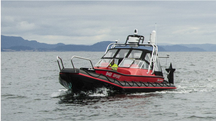
Figure 2. The Telemetron ASV, designed for both manned and unmanned operations. Courtesy of Maritime Robotics.
