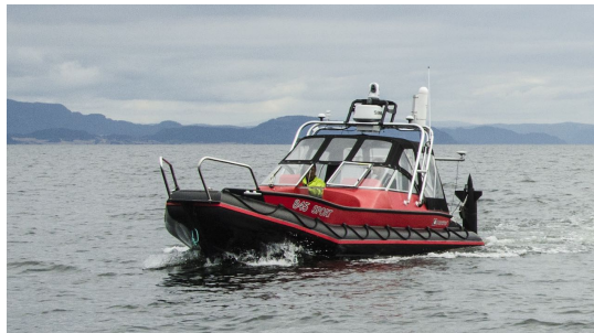
Figure 8: The Telemetron ASV, owned and operated by Maritime Robotics. Courtesy of Maritime Robotics.
