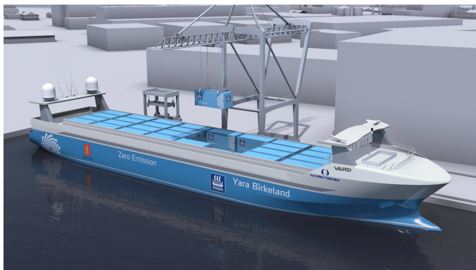
Figure 1.3: An illustration of the Yara Birkeland vessel, which is an example of a MASS. Courtesy of Marin Teknikk and Kongsberg Maritime.
