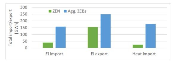
Figure 9.17: Total energy imports and exports for a ZEN and for the case of aggregated ZEBs
