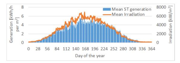
Figure 6.9: Daily mean ST generation and irradiation for one year
