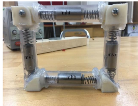
Figur 3.5: Tremor suppression with shape memory alloy vibration absorber
