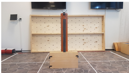
(e) Square steel pole placed on wooden box, supported by plastic half-pipe
