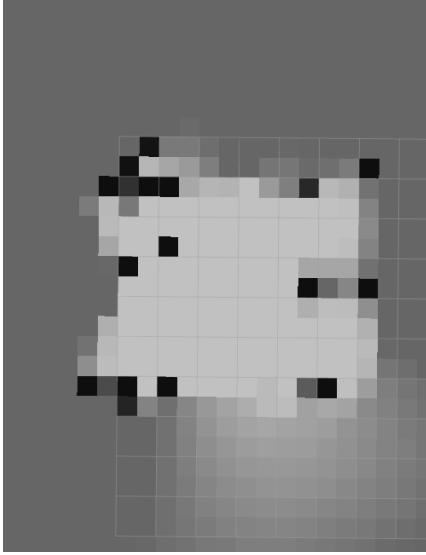
(a) Mapping of NTNU room with 0.5 meter resolution
