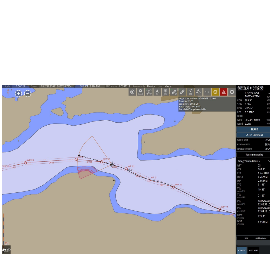
Figure 5.23: A screenshot of the simulated ship successfully following the route from figure 5.21.
