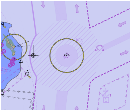
(a) Traffic separation scheme roundabout. The roundabout should be traversed counterclockwise.
