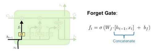
Figure 2.3.3: LSTM forget gate [23]
