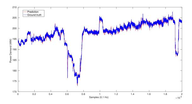
Figure 7.1.7: Power demand forecast using the squared version of trained readout weight
