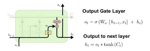
Figure 2.3.5: LSTM output gate [23]
