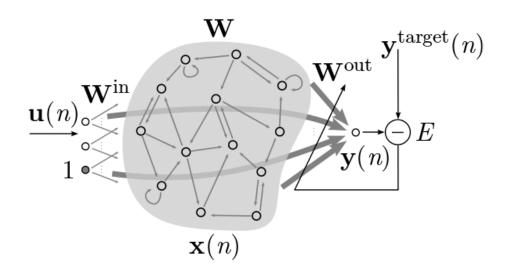
Figure 2.3.6: Illustration of the standard Echo State Network architecture
