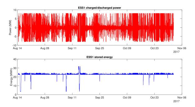
Figure 7.2.8: Charge/discharge rate and stored energy of ESS
