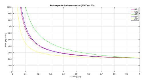
Figure 7.2.2: Brake Specific Fuel Consumption of the gas turbines normalized relative to the per unit loading
