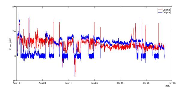
Figure 7.2.7: Optimal vs. original grid power when ESS is used
