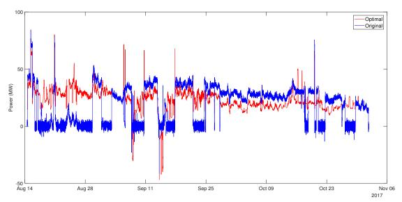
Figure 7.2.5: Optimal vs. original grid power with 5 MW as the grid power set-point
