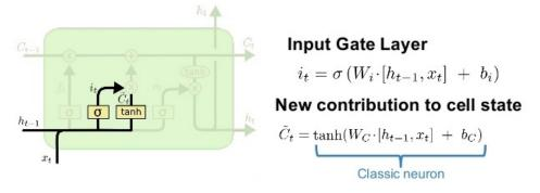
Figure 2.3.4: LSTM input gate [23]
