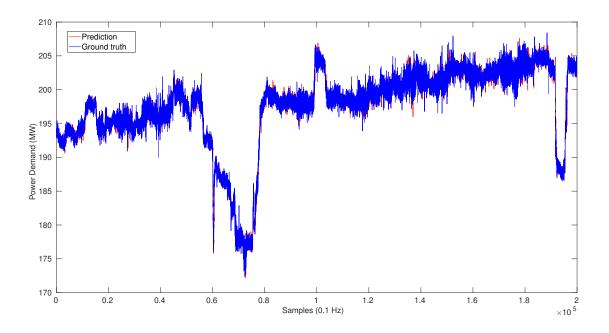
Figure 7.1.1: Power demand forecast using normalized test data
