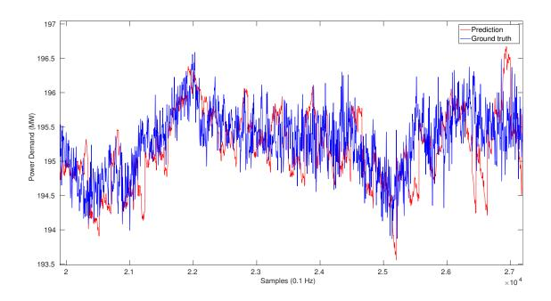
Figure 7.1.8: Power demand forecast covering sample sequence from 21000 to 27000 using the squared version of trained readout weight
