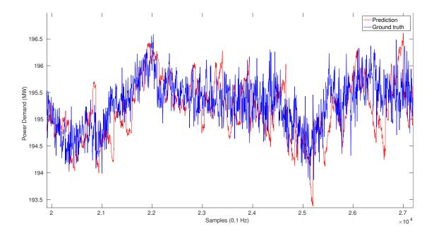
Figure 7.1.6: Power demand forecast covering sample sequence from 21000 to 27000 using the squared version of input vector
