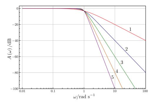
Figure 2.1.1: The gain of low-pass Butterworth filter with increasing order
