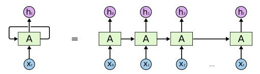
Figure 2.3.1: A simple feedback connection of RNN
