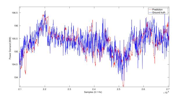
Figure 7.1.4: Power demand forecast covering sample sequence from 21000 to 27000 using the low-pass filtered and normalized test data
