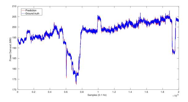
Figure 7.1.3: Power demand forecast using the low-pass filtered and normalized test data
