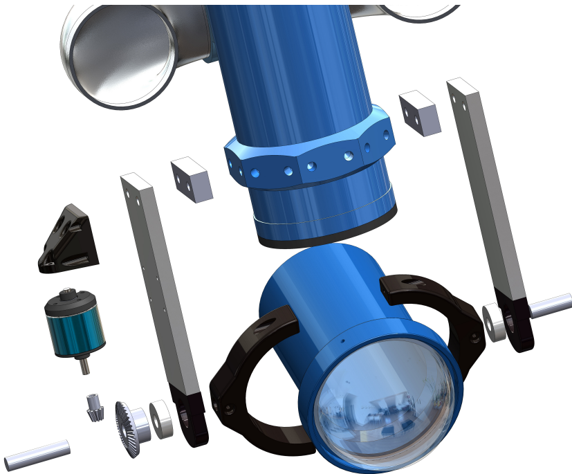
Figure 3.5: Pitch actuator, exploded view
