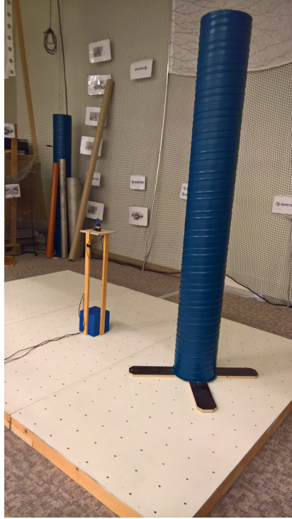
Figure 4.2: Test setup with one cylinder placed 0.92m away from the radar at 0^\circ .
