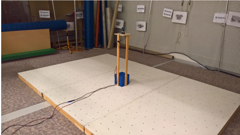
Figure 3.9: The test platform together with the pedestal on which the radar system was placed.
