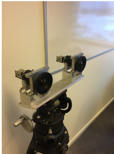
Figure 3.2: The stereo camera rig.
