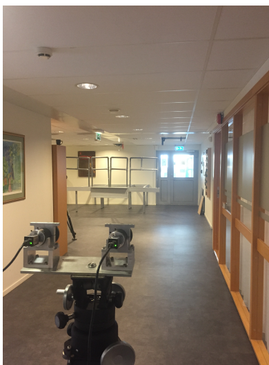
Figure 4.1: Taking images of the platform with the stereo camera at one of many locations.
