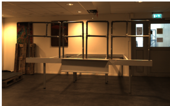
Figure 3.1: The platform built for experimental testing of the different algorithms and is a copy of an entrance of a windmill. The docking slot is positioned under the entrance in the center of the platform.
