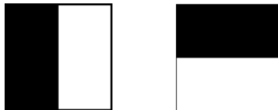
Figure 3.17: The Haar wavelet kernels used to compute the response in the horizontal (left) and vertical direction (right). The black and white regions have filter coefficients of -1 and +1 , respectively, [3].
