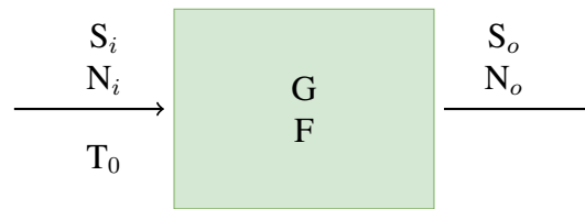
Figure 2.12: Relationship between the input and output in a two-port network.
