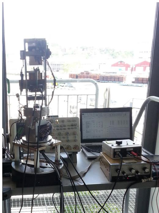
**Figure 4.1:** The fiber laser and APD mounted on the prototype.
