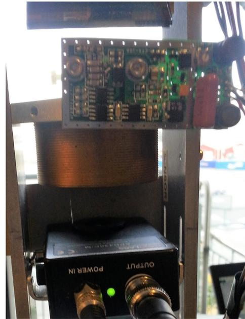
**Figure 4.3:** The diode laser and APD mounted on the prototype.
