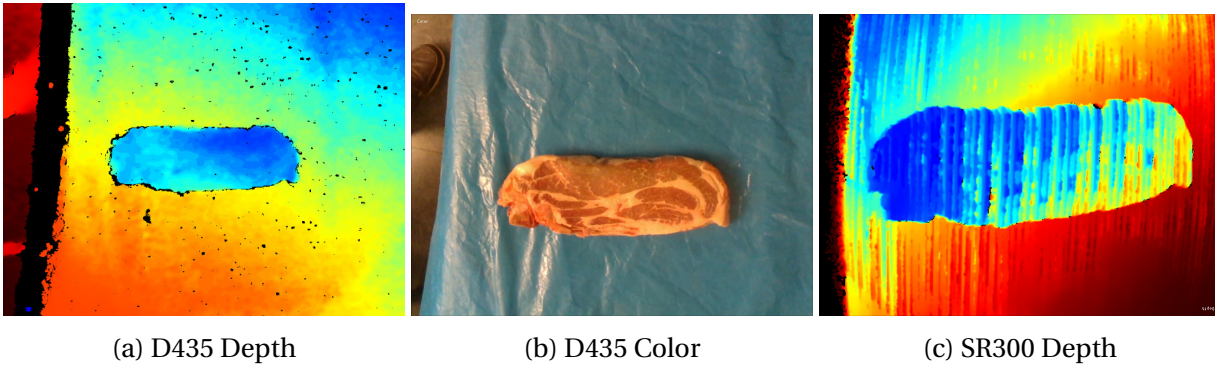
Figure 6.4: Figure showing some distortion artifact observed using the SR300 camera. (a) shows a depth image of a pork chop using the Intel RealSense D435 camera, (b) shows the same object with the color camera of the D435 camera and (c) shows a depth image of the same object using the Intel RealSense SR300 camera. The images are screenshots from the rs-capture tool provided with the Intel RealSense software ( Intel (2018a) ).
