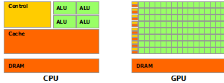
Figure 2.10: Figure showing a simplified architecture of a CPU (left) and a GPU (right) based on the die area. The figure is showing two architectures with the same die area, where the CPU typically dedicates more space for advanced control (more advanced instructions) and memory control (for more advanced memory accesses), while the GPU will dedicate more space to the arithmetical units. This enables massive parallelism for the GPU, while the CPU is better for serialized tasks and advanced branching patterns. The figure is taken from NVIDIA (2018) .
