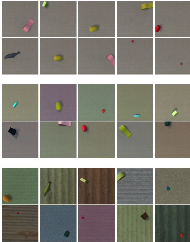
Figure 4.6: Examples of RGB visual observations from our simulation environment, where the depth images are omitted as they are mainly black in the first step of an episode. The first two rows show visual observations without DR applied, the two middle rows show visual observations with a Domain Randomization (DR) factor of 0.5 and the last two rows show visual observations with a factor of 1.0. As can be seen in these images, many aspects of the observations are randomized as the power of randomization increases.
