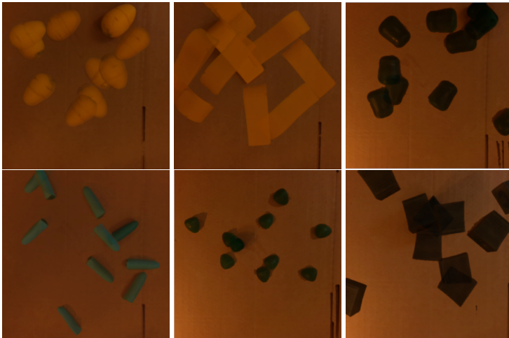
Figure 5.12: Visualization of the ten random initial configurations for each object used in our real world experiments. For each object, each unique position and rotation is shown per image, visualizing the distribution of our test set. The objects shown are respectively left to right, top row; Avocado, Fish Fillet and Paprika, bottom row; Pickle, Strawberry and Speaker.
