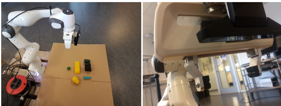
Figure 4.8: Photographs showing our real world setup for the gripping pose estimation problem, with the Panda robot by Franka Emika (Franka Emika, 2018a) and a RealSense SR300 camera (Intel, 2018) mounted on its end-effector.
