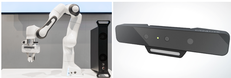
Figure 4.7: The Panda robot by Franka Emika in a real world setup (Franka Emika, 2018a) and the Intel RealSense SR300 depth sensing camera (Intel, 2018), both shown untethered.
