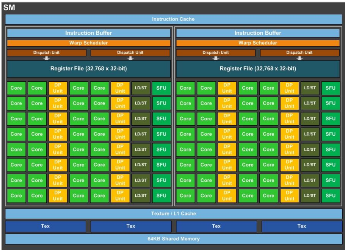
Figure 2.3: Architectural overview of a single SM in the Pascal GP100 GPU. From NVIDIA Tesla P100 [30] with permission.
