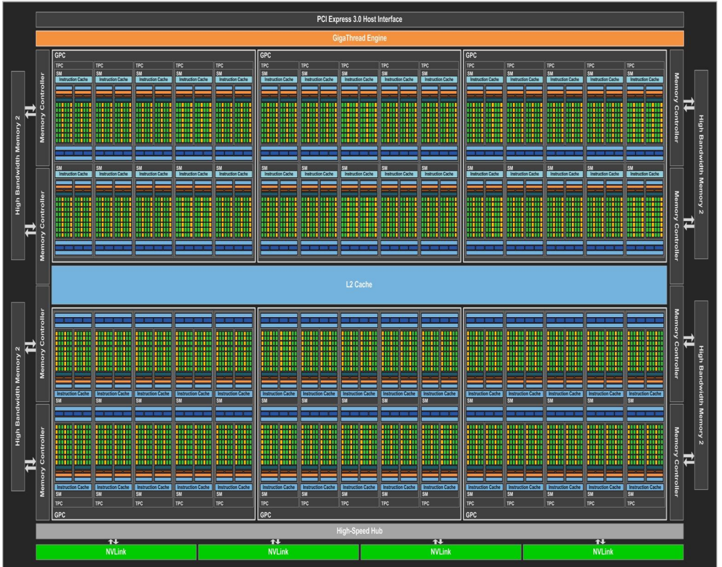
Figure 2.4: Architectural overview of the Pascal GP100 GPU found in the NVIDIA Tesla P100. From NVIDIA Tesla P100 [30] with permission.
