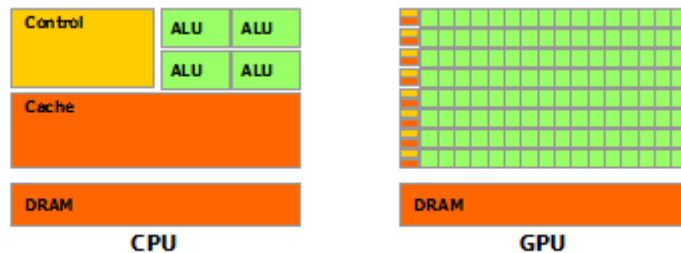
Figure 2.1: Comparison of how transistors are used in a CPU compared with a GPU. From CUDA C Programming Guide [7] with permission.
