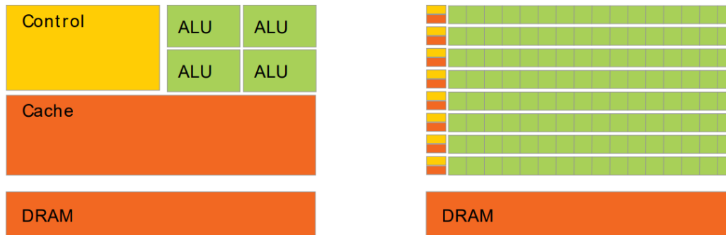
Figure 2.1: The difference in hardware on the CPU and on the GPU, focusing on the distribution of DRAM, cache, control units, and ALUs for each device. From CUDA C Programming Guide [35] with permission.
