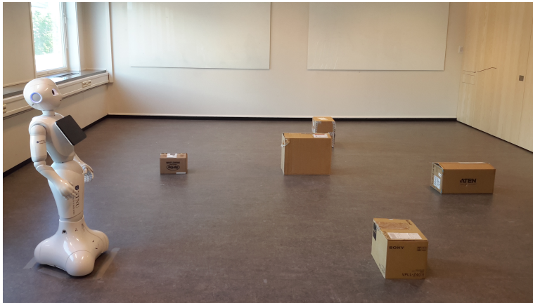
Figure 4.2: The area prepared for Pepper to perform a navigation task with obstacle avoidance.
