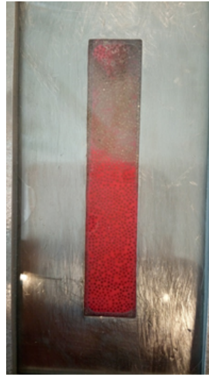
Figure 5.8: Creaming due to high porosity of the cell
