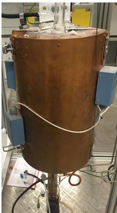
(a) Calsination reactor in the tubular oven.
