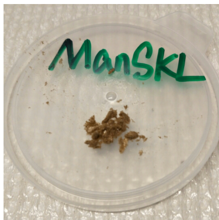
Figure 3.11: The ManSKL sample after freeze drying, with light brown color and fluffy structure.
