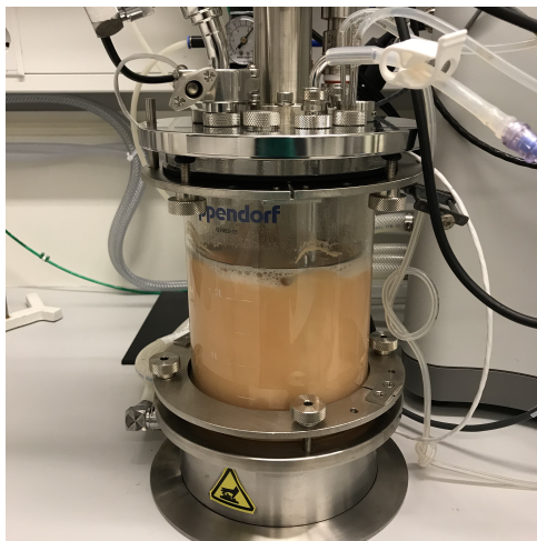
FIGURE 2.8: Bioreactor culture of Aurantiochytrium sp. T66. The characteristic orange color induced by astaxanthin and carotenoid production become very clear during lipid accumulation.
