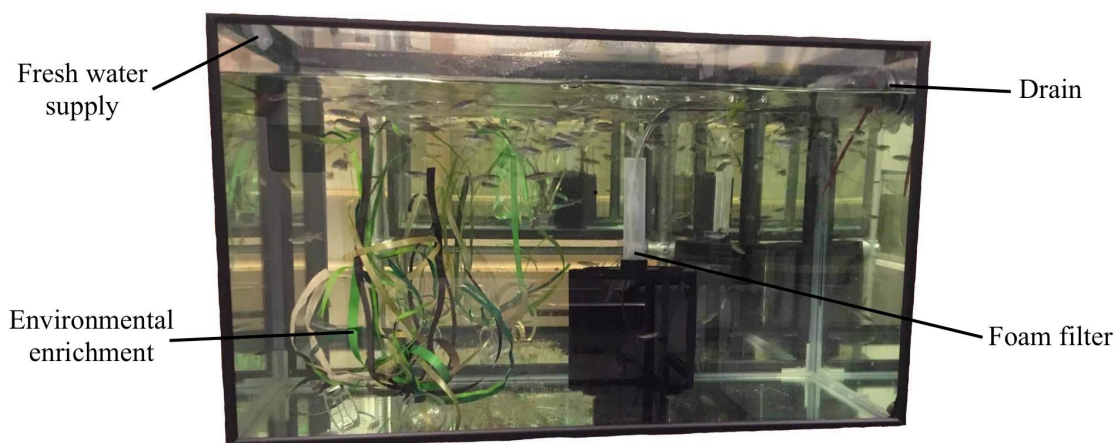
Figure 3.1 Tank setup with fresh water supply, environmental enrichment, drain and foam filter
