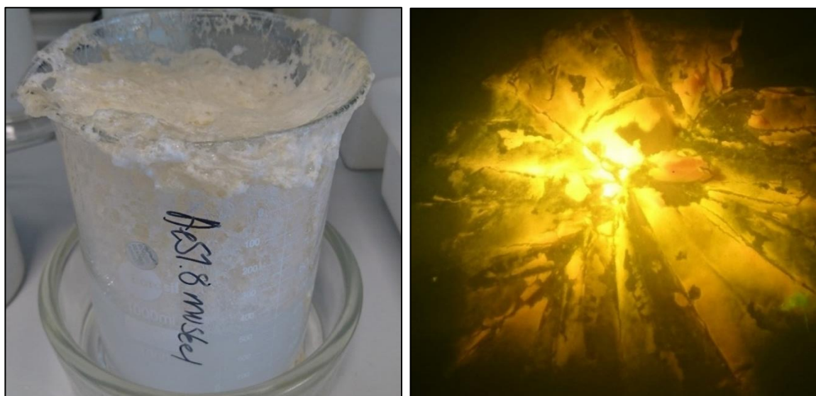
Figure 2.3-1: Left: Formation of foam during digestion of muscle tissue. Right: Typical view of filters from muscle samples through light barrier filter, no microscope magnification.
