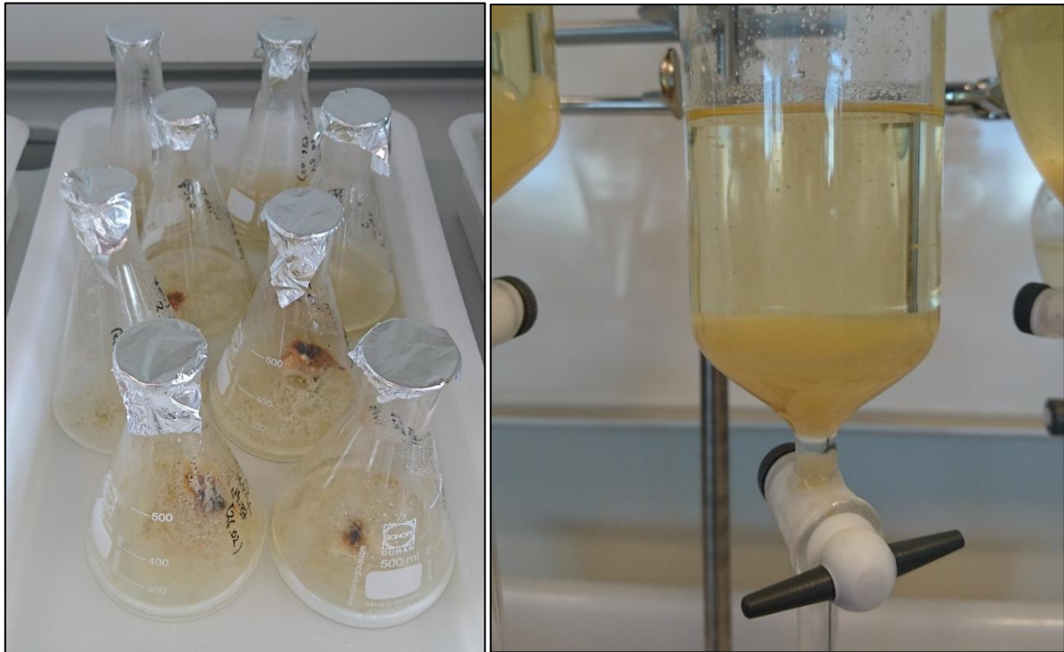
Figure 2.2-2: Left: Digestion of stomach tissue, early phase. Right: Density separation of digested muscle tissue using separation flasks. Picture taken after 3:30 hours of sedimentation. Photo: Ådne Messel Nafstad
