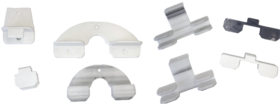
Figure 5.10: Picture of various iterations of the simplified gripper tooling for manipulator testing.
