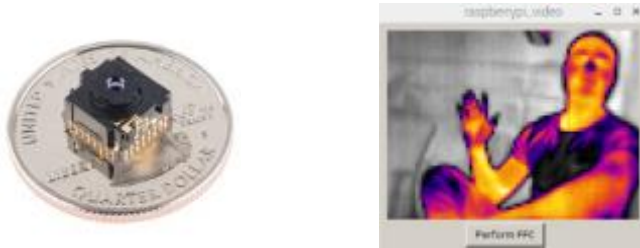
Figure 36: FLIR Lepton camera module and Raspberry Pi video test output
