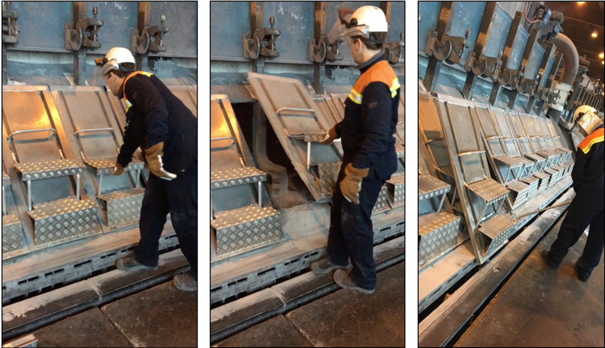
Figure 3.5: A process engineer at Alcoa Mosjøen performing typical handling of pot covers.
