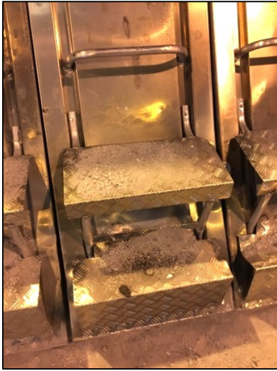
Figure 3.10: Dirt and dust covering the pot cover step surfaces.
