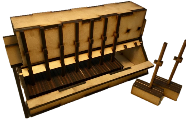
Figure 2.2: Communicative prototype of a smelting pot with detachable anodes.
