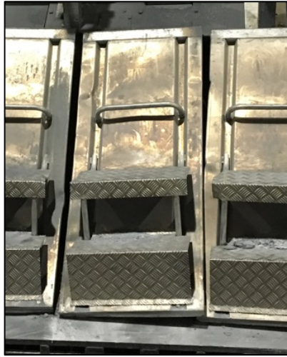
Figure 3.13: Misplaced pot cover, resulting in crookedness and a gap between covers.
