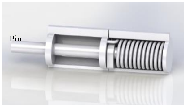
Figure 9: Spring loaded hinge pin, enclosed (right) and cross-sectional (left). The front section contains the torsion spring, accumulating torsional energy between the front and rear section. The rear section contains a chamber available for potential viscous or friction dampening designs. The design is purely mechanical for better coping with the harsh environment.
