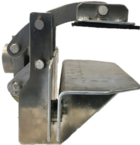
Figure 4.26: Side view of the final gripper prototype. Detailed viewing of the step plate slot, support bracket and step plate support surface.
