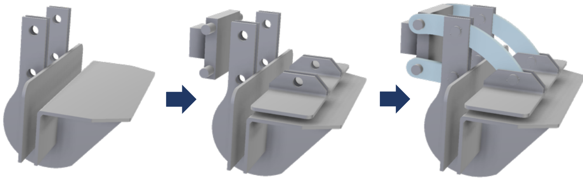
Figure 4.23: Pictures depicting the approach for the linkage design. First, the rigid part of the tool was modelled, with holes for the bearing rods. Secondly, placement of the clamping plate and manipulator connection bracket was inserted. From the restricting dimensions created from the two first steps, links joining the prehension mechanism components was made.
