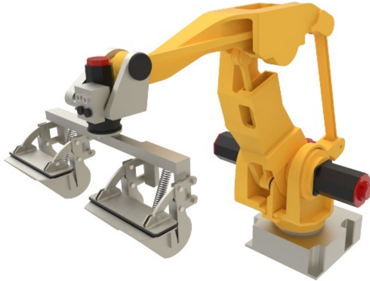
Figure 6.11: Visualisation of the proposed robot solution installed with the gripper tool concept. A small gripper design modification is performed to allow connection with the robot. The yellow robot is a model of the FANUC M-420iA robot acquired from GrabCAD (TheNicman 2017).
