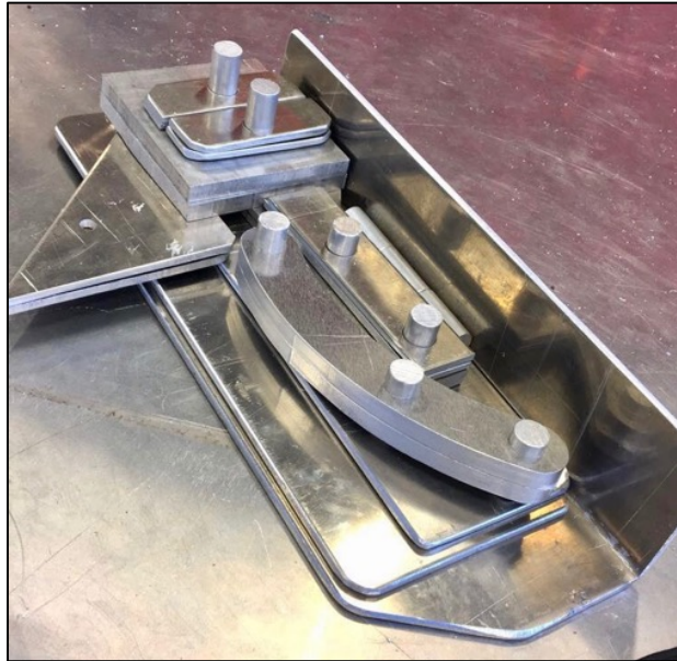
Figure 4.24: All subcomponents of the final gripper prototype gathered before welding assembly.
