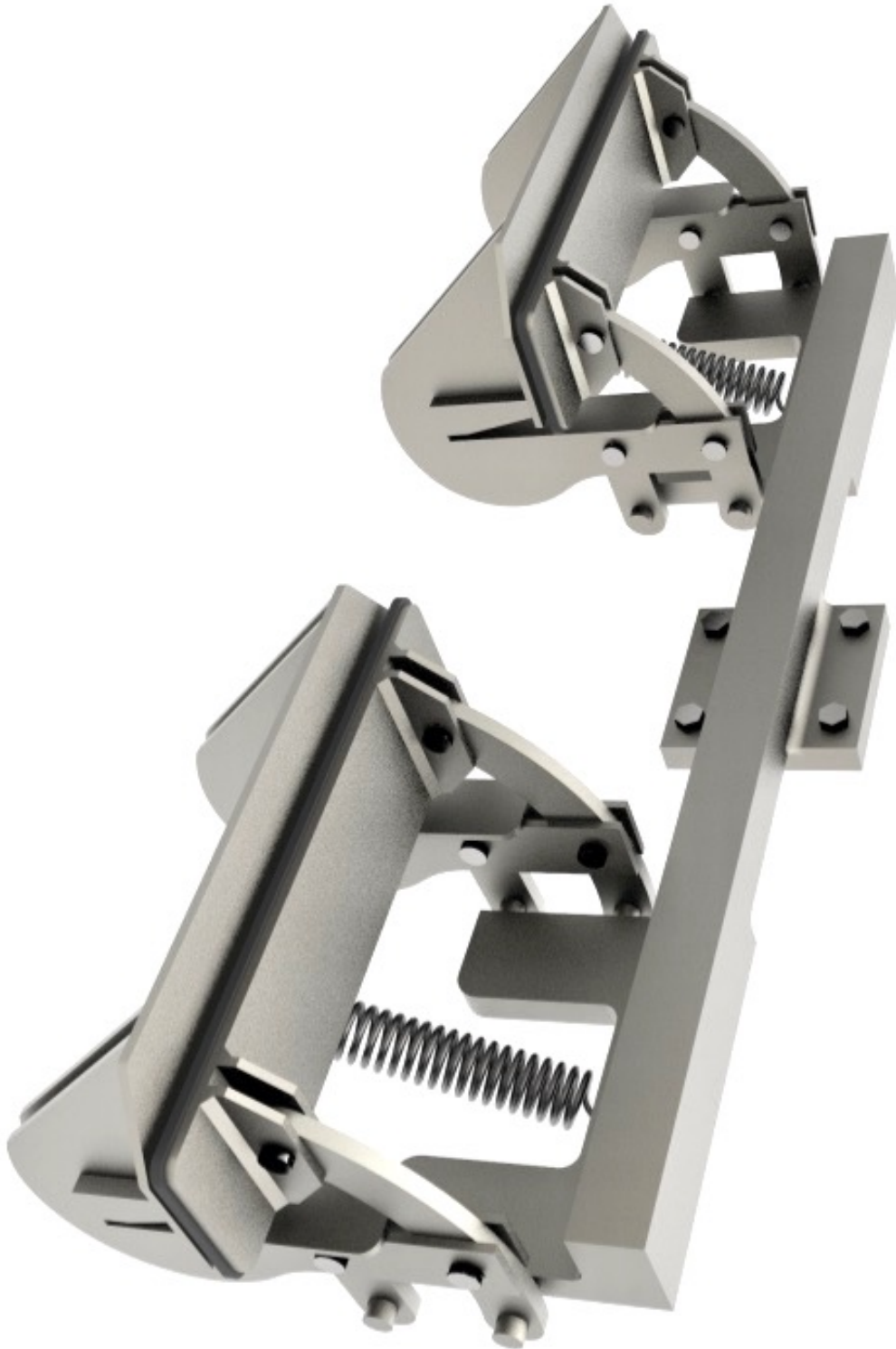
Figure 10.1: Isometric HQ render of the final iteration dual robot gripper.
