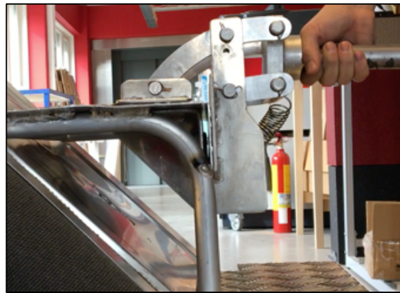
Figure 4.31: Fourth step of gripping: Raising the robot arm, the clamping mechanism activates. Gradually, the cover becomes increasingly restrained until force match occurs and the cover can be handled.
