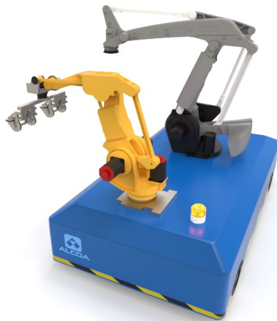
Figure 6.12: Visualisation of the proposed robot system on a mock-up AGV. The grey robot is a placeholder for the anode covering robot acquired from GrabCAD (Bejenaru 2017; TheNicman 2017).
