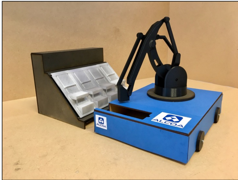
Figure 5.7: Picture of the ready-for-use feasibility test setup, containing a pot section with four pot covers and a mobile AGV platform. A 3D-printed mock-up robot is added to the AGV, representing the anode covering robot.
