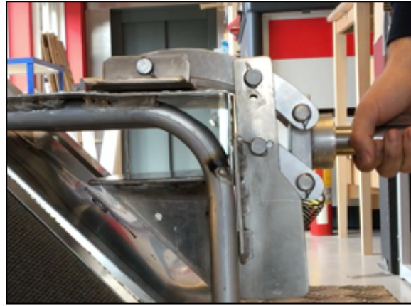
Figure 4.29: Second step of gripping: The tool is inserted until it reaches the gripper abutment
