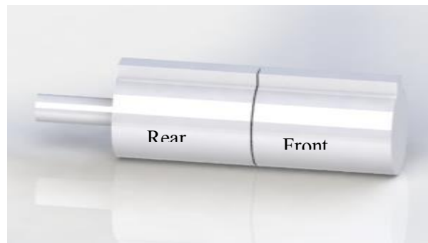
Figure 9: Spring loaded hinge pin, enclosed (right) and cross-sectional (left). The front section contains the torsion spring, accumulating torsional energy between the front and rear section. The rear section contains a chamber available for potential viscous or friction dampening designs. The design is purely mechanical for better coping with the harsh environment.
