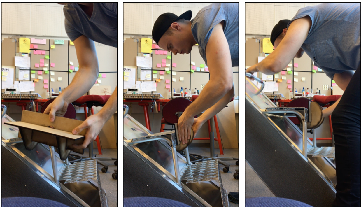
Figure 4.18: Pictures captured during the critical function testing of the third iteration gripper prototype. The pictures depict insertion and cover lifting with the concept.
