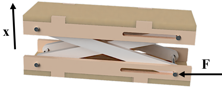
Figure 5.14: Rendered detailed view of the scissor mechanism CAD assembly. Exerting force on the bottom link bar will result in elevation of length x of the lift table.
