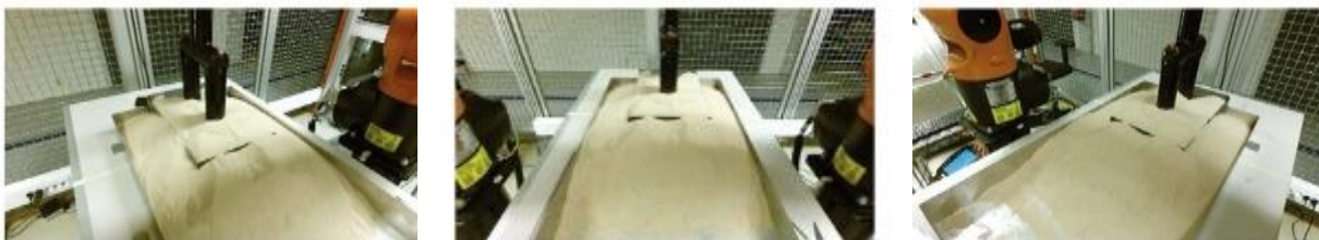
Figure 16: Anode covering mock-up. Centred view and +35° side views from Kinect.
