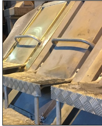
Figure 3.14: Differences between pot cover handlebar height.
