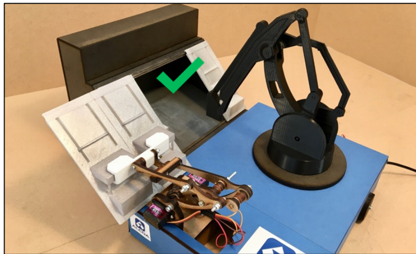
Figure 5.22: Pictures showing the successful testing of the Articulated manipulator concept. Having already aligned the AGV, the top left shows the AGV aligned and the manipulator ready for gripping of the two pot covers. The top right picture shows the manipulator after accomplished cover handling. By driving the AGV along the pot, the pot operation robot gains free access to the inside of the pot, depicted in the bottom picture. Video link in appendix A.
