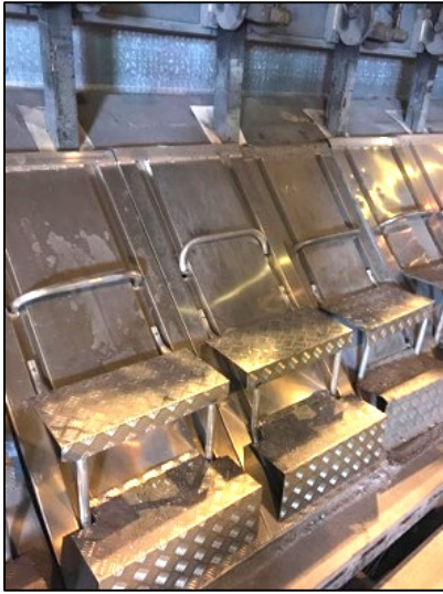
Figure 3.7: Pot cover with the handlebar torn off.
