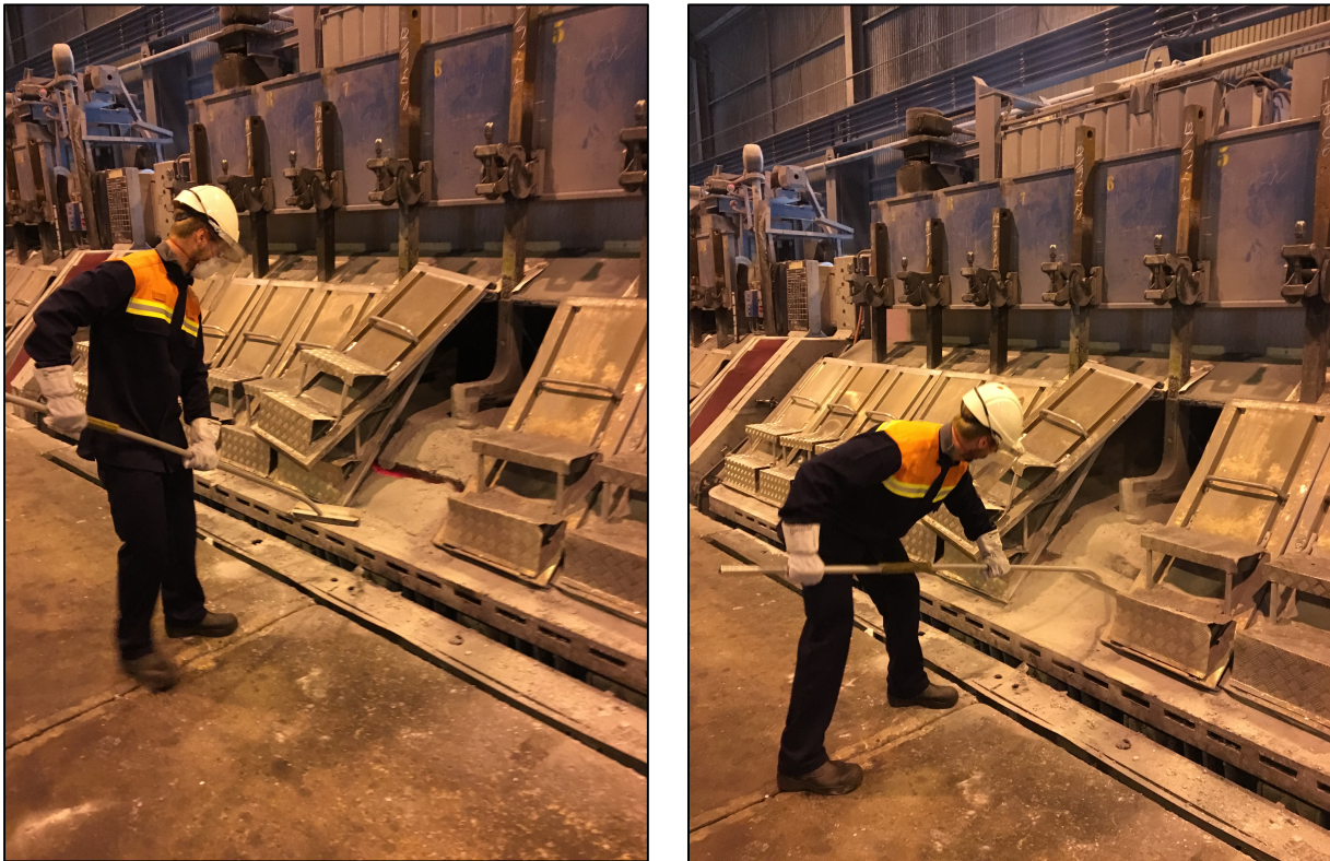
Figure 1.2: The manual operation of anode covering being performed at Alcoa Mosjøen.
