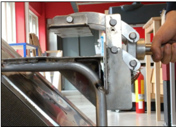
Figure 4.30: Third step of gripping: The EOT is raised vertically, achieving front plate slot insertion and tool contact with the step plate surface.
