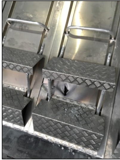
Figure 3.8: Pot cover with a severe tear.
