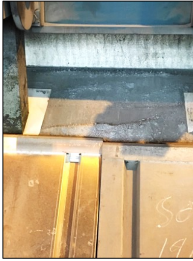
Figure 3.11: Dirt and dust are resting on top of the smelting pot cover rack.
