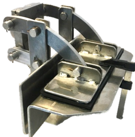
Figure 4.25: Isometric view of the proof-of-product prototype. An F-clamp is used to hold the clamping mechanism shut, as it is normally open due to the spring.
