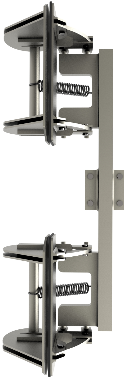
Figure 10.2: Front view HQ render of the final iteration dual robot gripper.
