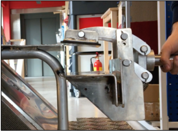
Figure 4.28: First step of gripping: The gripper is centralised and aligned for insertion underneath the second step.
