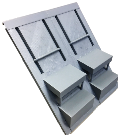
Figure 4.2: Simplified pot covers 3D-printed in PLA, made for ideation session.
