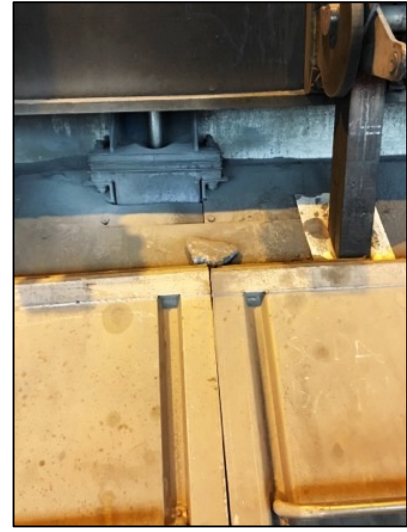
Figure 3.12: Chunks of solidified cover mass rest on top of the smelting pot cover rack.
