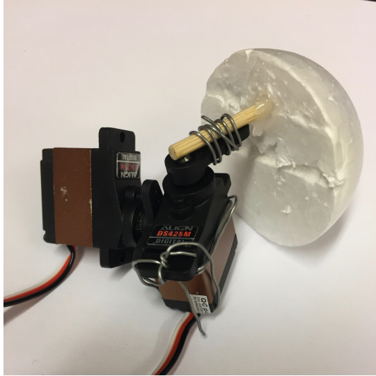
Figure 4.4: Simple mechanical actuation with two servo motors.
