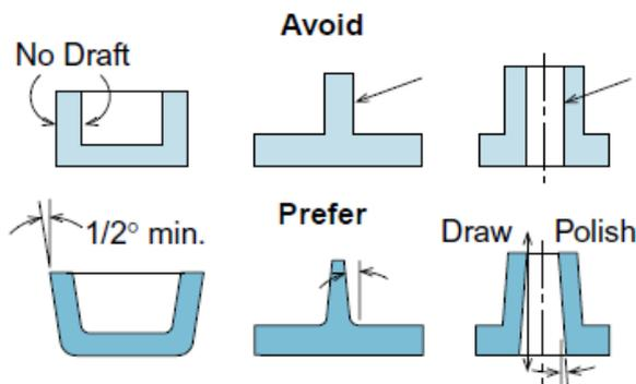
Figure 10 - Draft angles. Retrieved from *Part and Mold Design* (2016)
