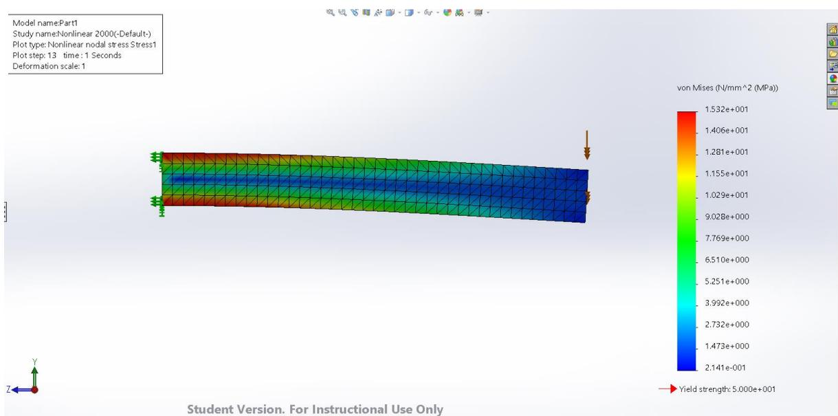
Figure 56 - Non-linear beam analysis
