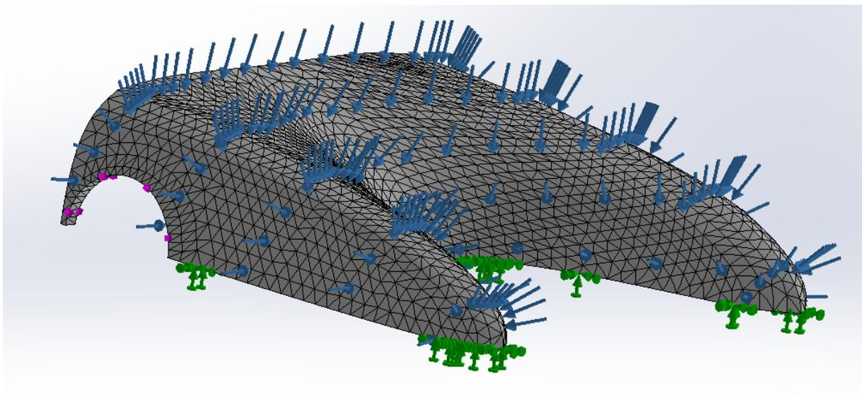
*Figure 59 - Boundary conditions in FEA of side cover*
