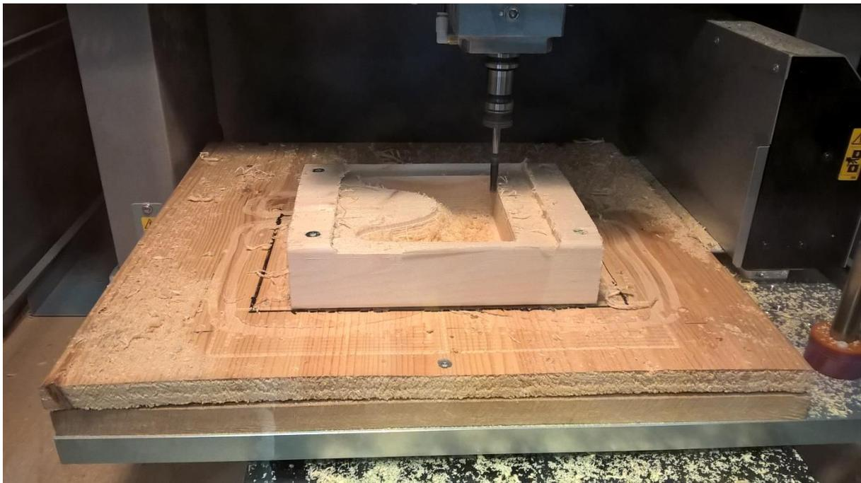
*Figure 22 - Milling of wood mold*
