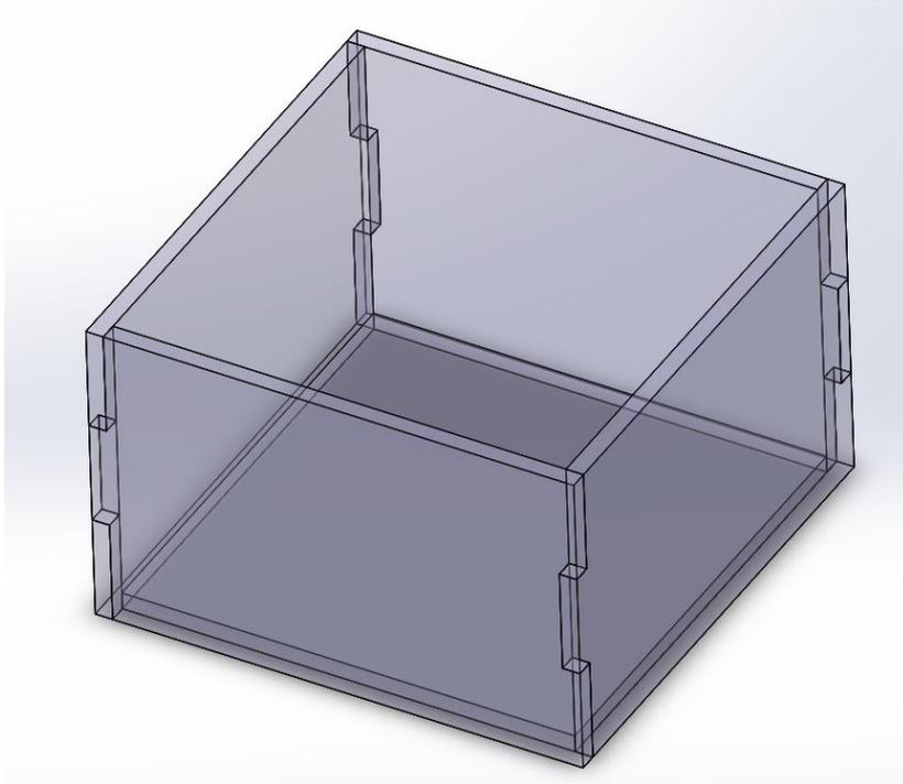
*Figure 25 - Silicone casting box*
