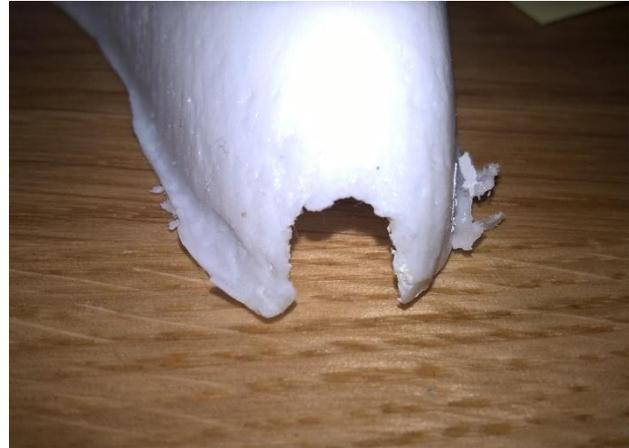
*Figure 37 - Damages from ejection*
