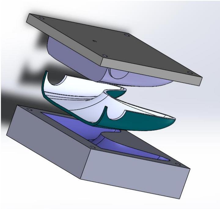
*Figure 21 - Assembly of molds with casted part*
