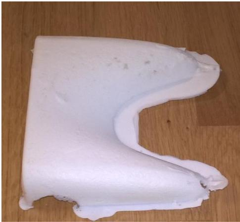
*Figure 38 – Excess material*
