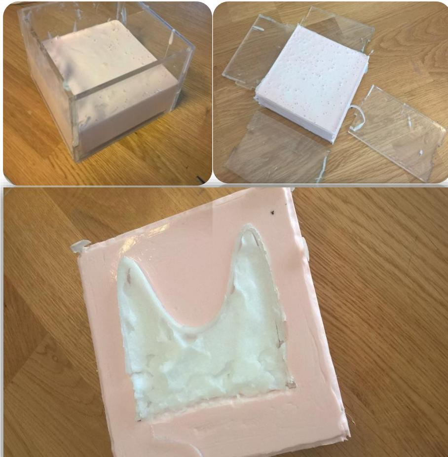
*Figure 26 - Image series of casting of silicone mold*
