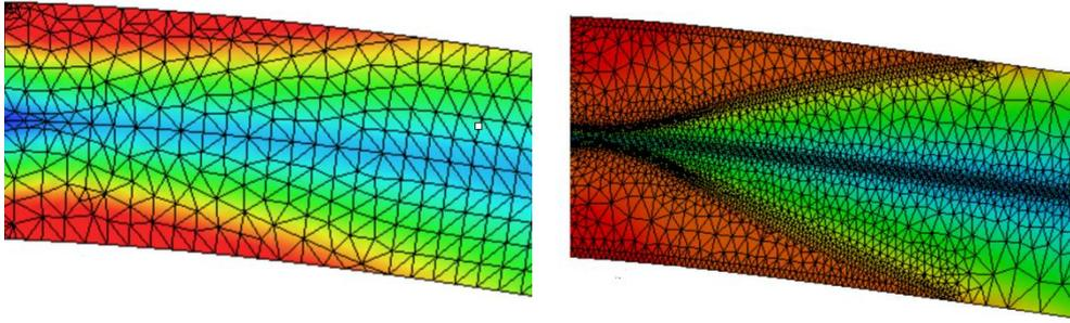
Figure 57 - Stress distribution in critical area. Linear test to the left and non-linear test to the right at 2000N load.
