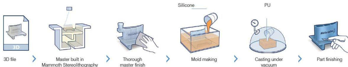
Figure 8 - Vacuum casting process. Retrived from Materialise (2016).
