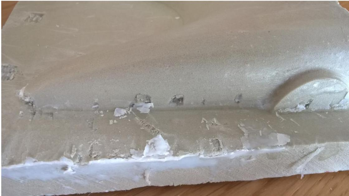
*Figure 42 - Damages after using screwdriver*
