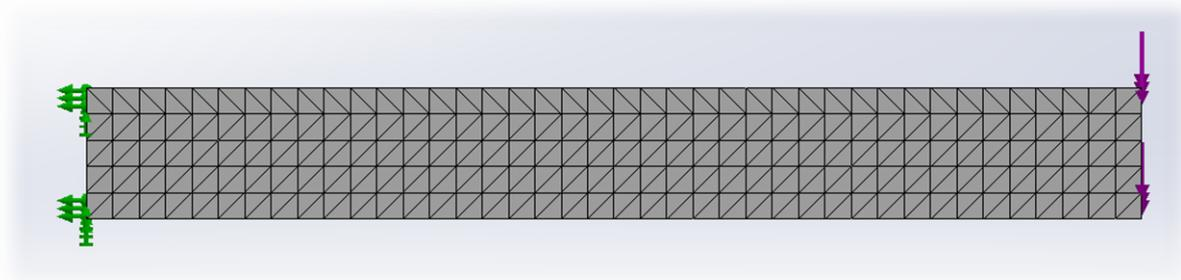
Figure 54 - Boundary conditions beam test
