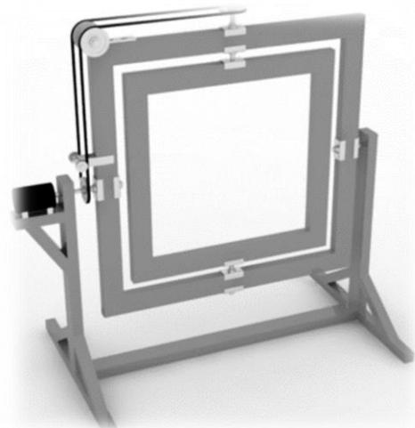
*Figure 7 - Frame for rotating molds when curing, designed in SolidWorks*
