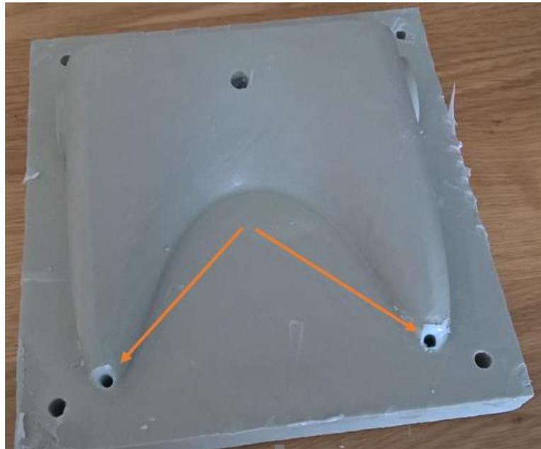
*Figure 35 - New inlet gates*
