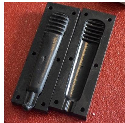
*Figure 29 - Good result with injection molding*
