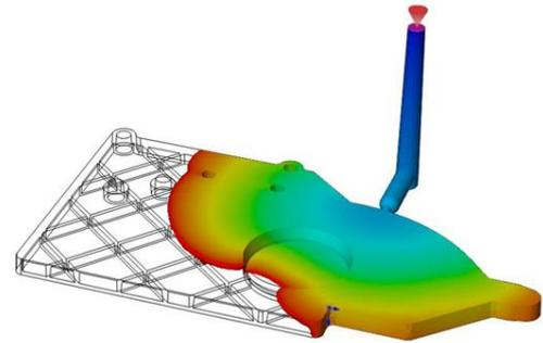
Figure 5 - Filling from injection molding.
