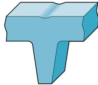
Figure 12 - Sink Marks. Depicted from *Part and Mold Design* (2016)
