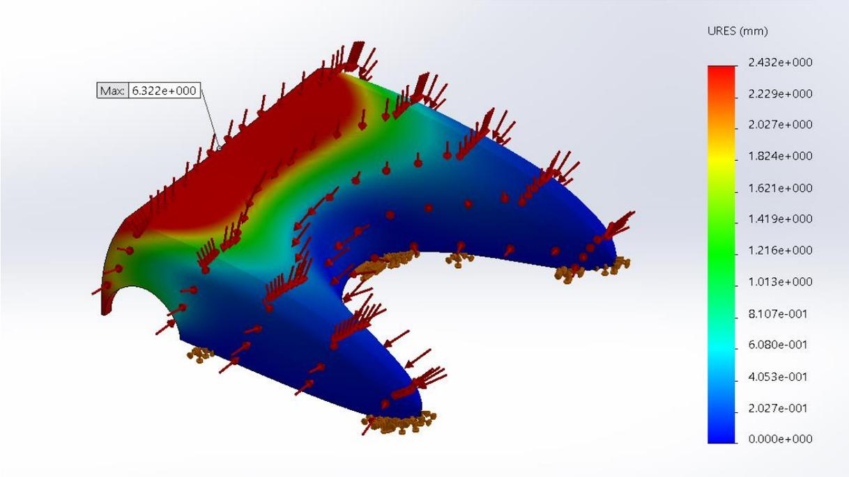
Figure 63 - Displacement standard model
