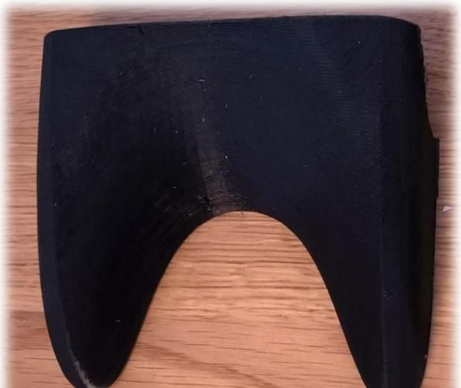
Figure 47- Layers from 3D-printing
