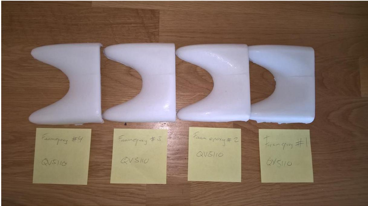
Figure 39- Models from foam-epoxy mold
