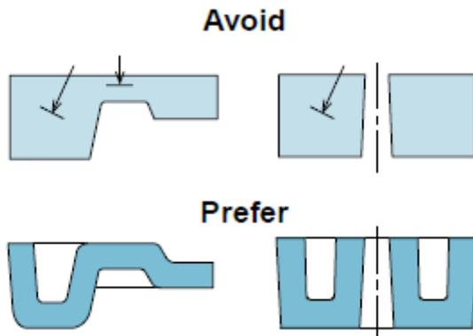
Figure 9 - Uniform wall thickness. Retrieved from *Part and Mold Design* (2016)
