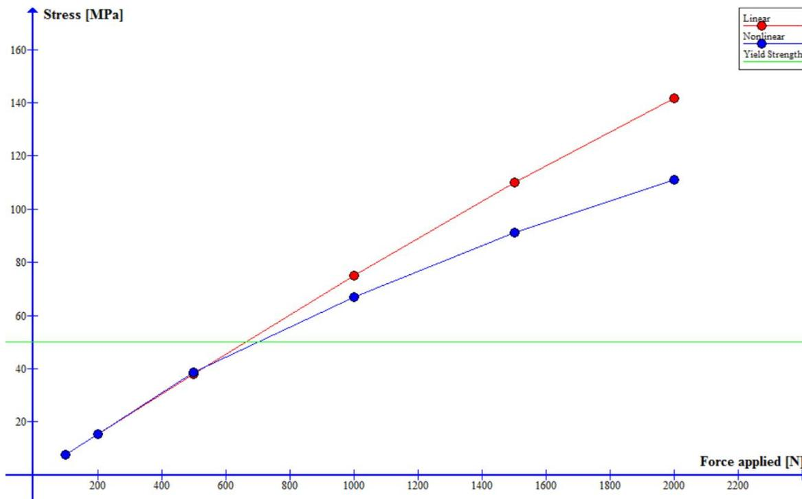
Figure 58 - Linear vs non-linear approach
