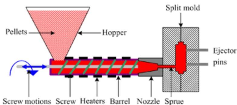
Figure 6 - Principals of an injection molding facility. Retrieved from <http://www.veejayplastic.com/>
