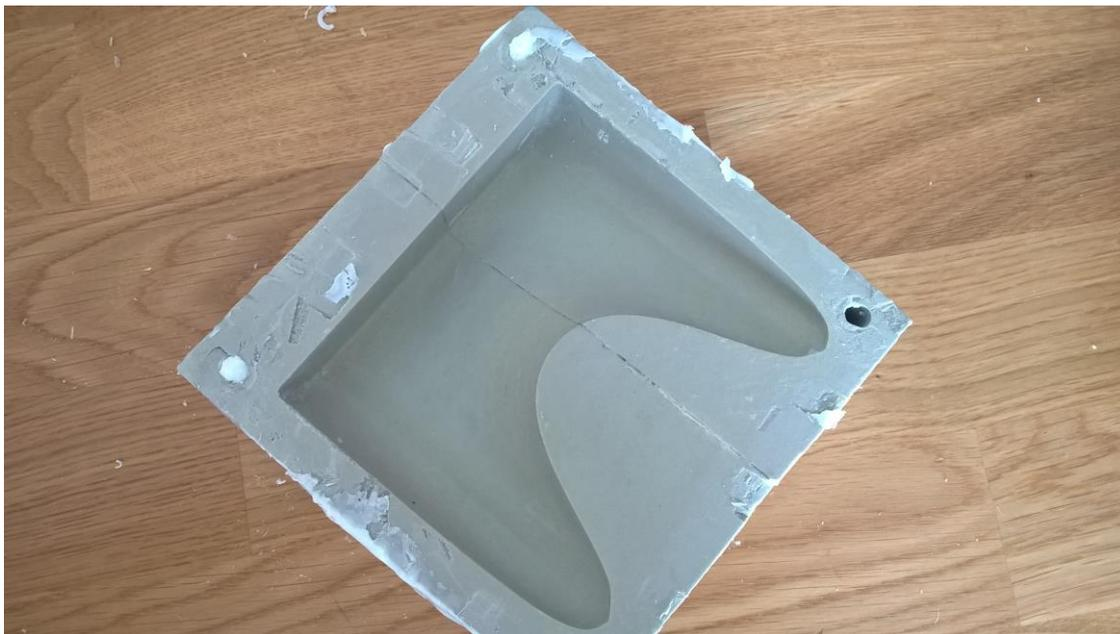
*Figure 43 - Wear of foam-epoxy mold*
