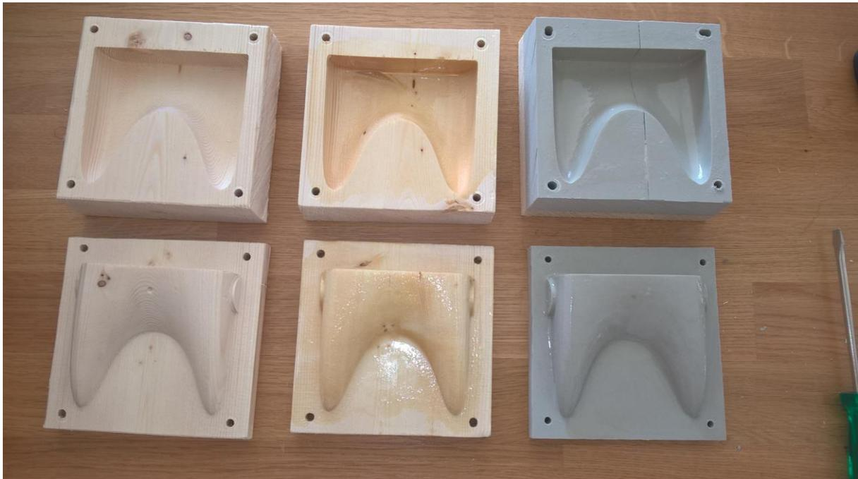
*Figure 33 - Surface treatment (wood, wood-epoxy and foam-epoxy)*
