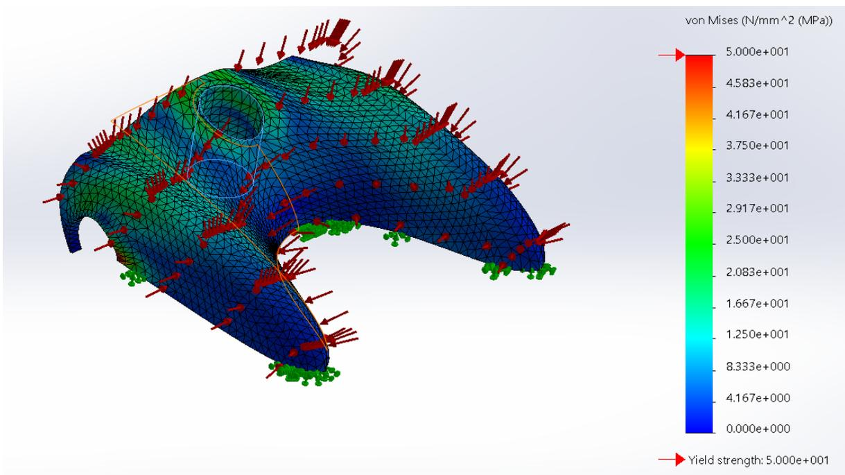
Figure 62 - Stresses rib model
