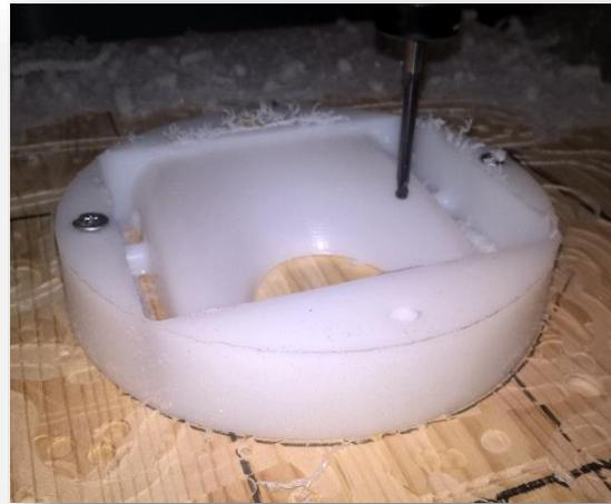
Figure 44 - Milling of prototype
