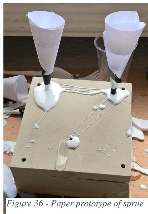
*Figure 36 - Paper prototype of sprue*
